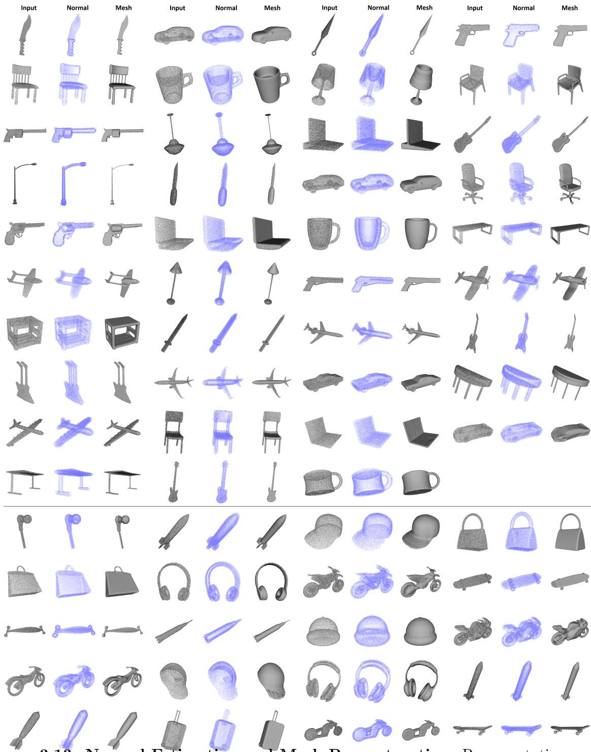
Figure 3.13: Normal Estimation and Mesh Reconstruction. Representative results of point cloud normal estimation and Poisson mesh reconstruction on the ShapeNet dataset. We test on input point clouds that have 8192 points though our method, POF, is trained using point clouds with 2048 points. Held-out samples from the ShapeNet training categories are above the line and leftout categories are below the line.
