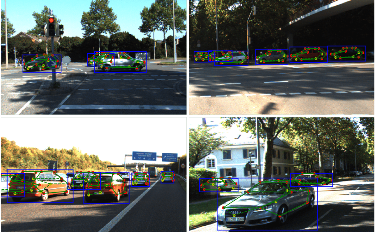
Figure 2.1: Representative 3D detection results, shown as projections on the input images. 3D morphable shape models of each vehicle are colored in green. Dashed green lines are occluded edges. For the 14 vertices of each morphable shape model, visible vertices are colored in red and occluded ones in yellow. 2D bounding boxes are colored in blue.
