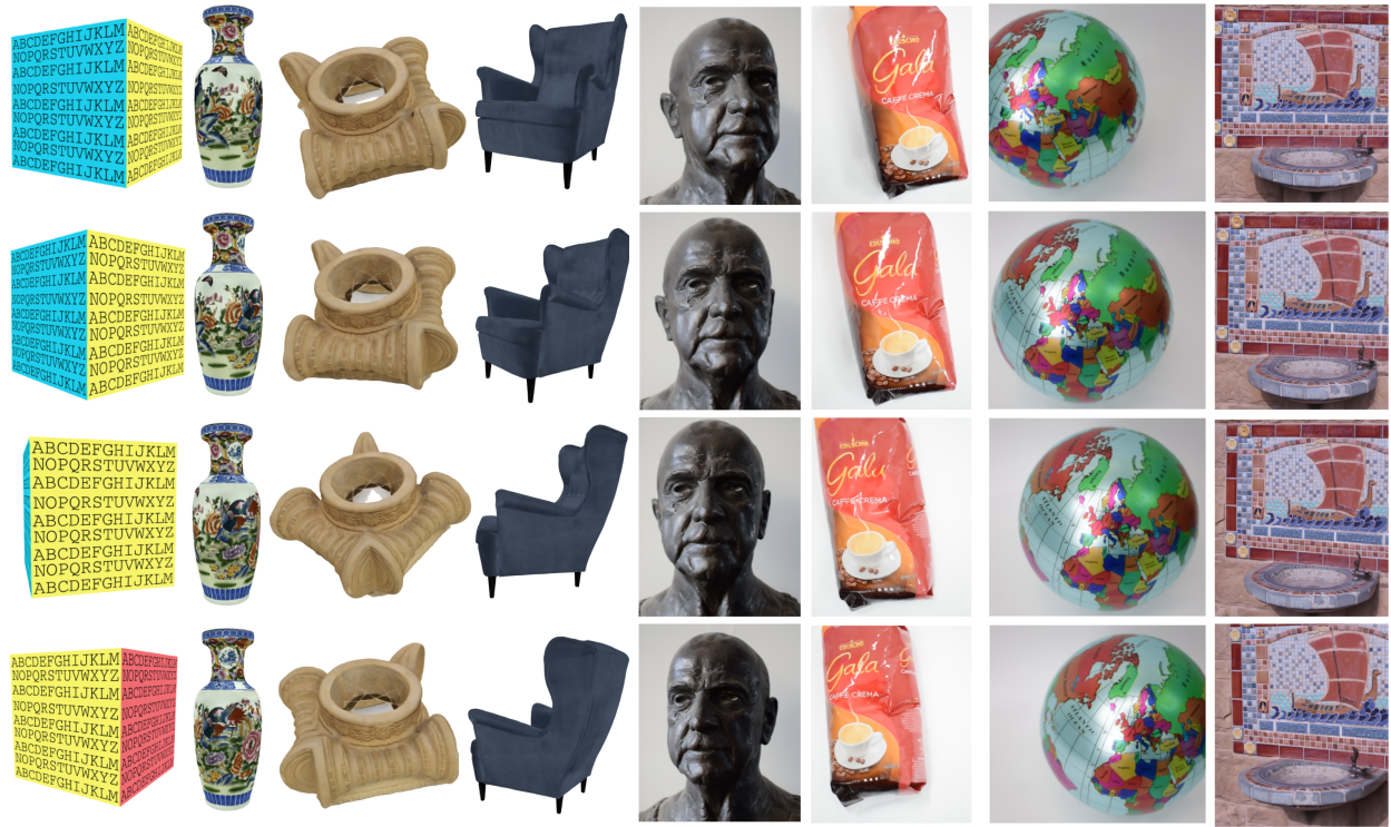
Figure 6.5: Novel-view synthesis results of DeepVoxels++ on objects with large viewpoint changes and complex shape/texture patterns. Our model is proposed for diffuse objects but we also show a few preliminary results on objects with specularities and shadows.
