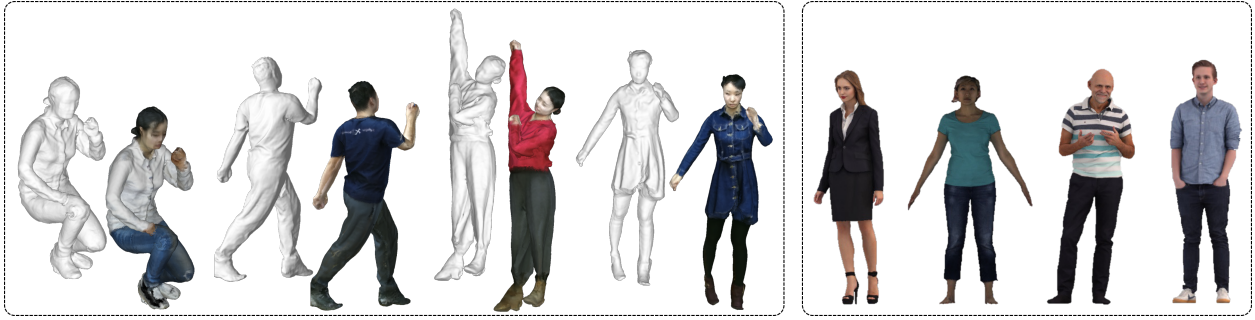
Figure 4.2: Left: the DeepHuman dataset contains various clothes and poses. Right: the dataset used in PIFu consists of mostly upstanding poses.
