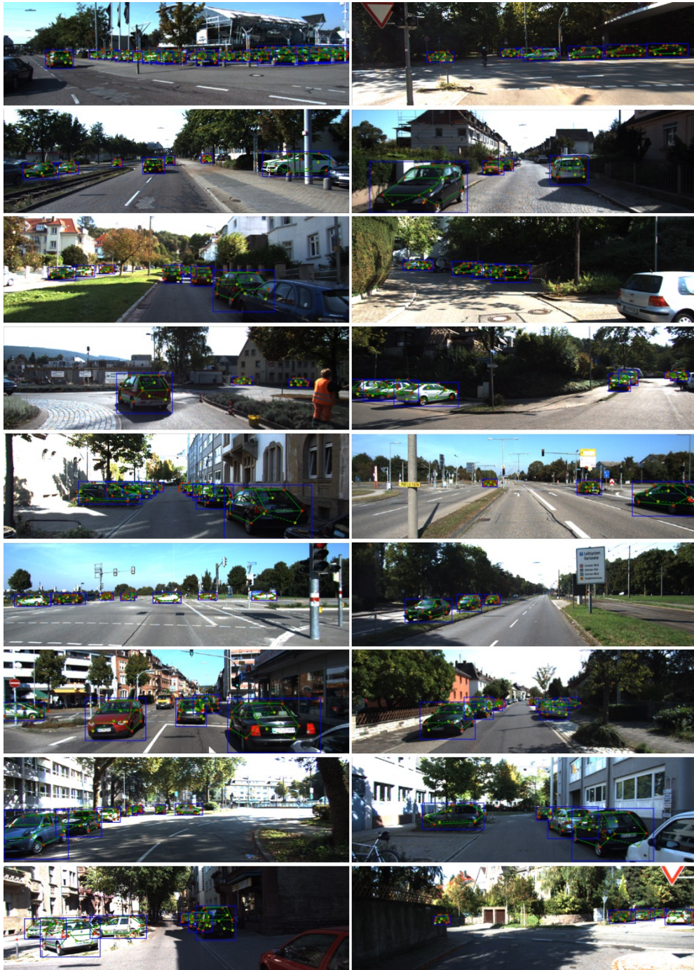
Figure 2.9: 3D detection results on KITTI test set, shown as projections on the input images. 3D morphable shape models of each vehicle are colored in green. Dashed green lines are occluded edges. For the 14 vertices of each morphable shape model, visible vertices are colored in red and occluded ones in yellow. 2D bounding boxes are colored in blue.
