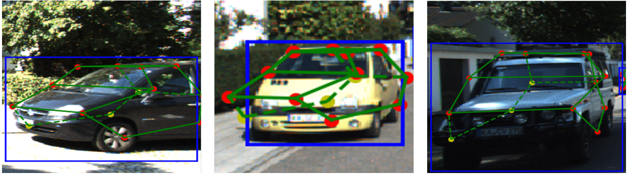
Figure 2.6: Failure cases caused by field of view truncation, inaccurate orientation or 3D scale estimation.
