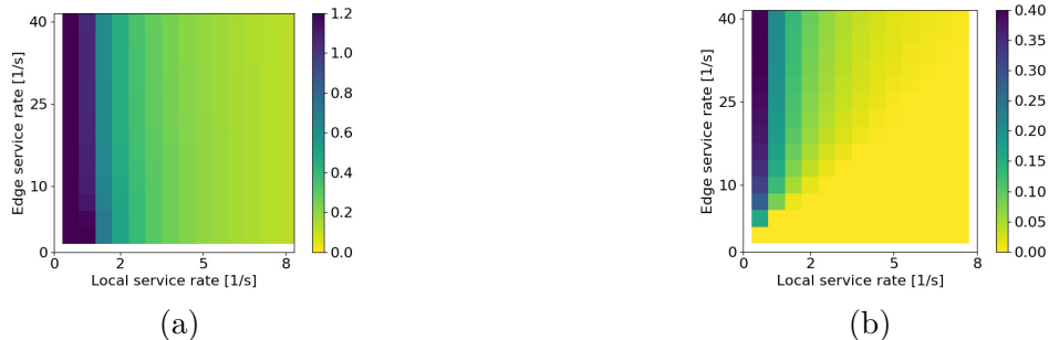
Figure 5.15: (a) Delay and (b) standard deviation for delay over a trajectory for different hardware configurations with average SNR of 16dB and no server load. Processing speeds are referenced as serving rates \mu .
