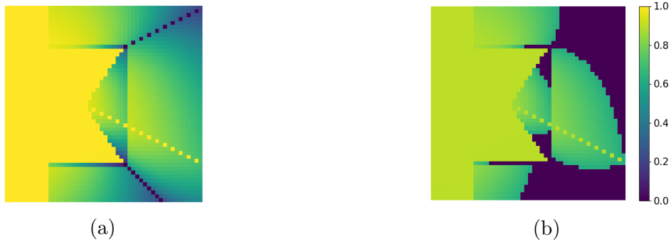
Figure 5.7: Offloading probability on the considered map. The average SNR is set to 9dB and server load set to (a) 0% and (b) 70%.
