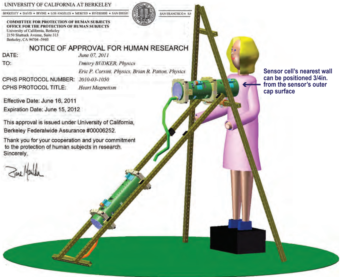
Figure 4.14: Another possible configuration to measure the magnetic field from the heart. In the above configuration the alkali cell's wall is positioned 3/4 in from the human subject's skin surface. Human research approval was obtained from the Office for the Protection of Human Subjects; the approval is renewed yearly. A measurement has not yet been realized. [Conception/design/construction (2006-08): E. Corsini - P.I.: D. Budker]
