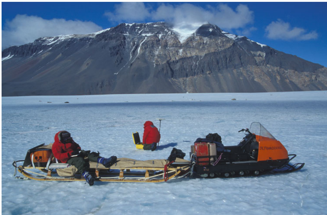
Figure 2.7. A typical ablation pole installation. Here Jeff and Kurt were measuring the pole's position with GPS, and making notes about the character of the glacier surface. Picture by Andy Bliss.
