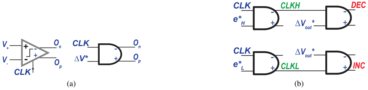
Figure 7.10: Quantized gate-level implementation. (a) Equivalence of a clocked comparator to a quantized AND gate. (b) Quantized gate-level implementation of the PD compensator truth table in table 7.2.
