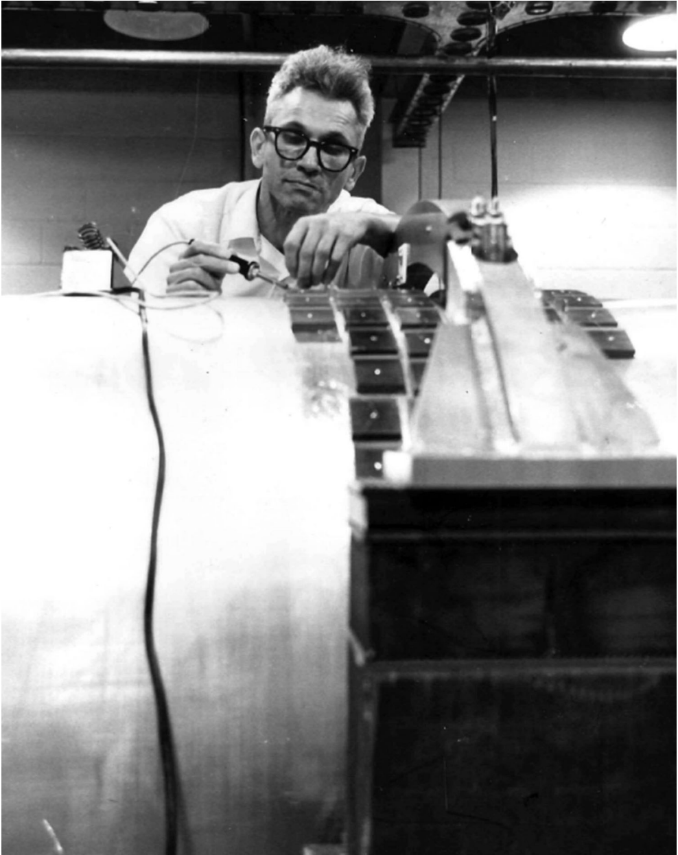
Fig. 4. One of the several standard images of Weber posed as if working on a bar antenna, either gluing on crystals or soldering them to wires that would connect to the outside. Probably 1969.
