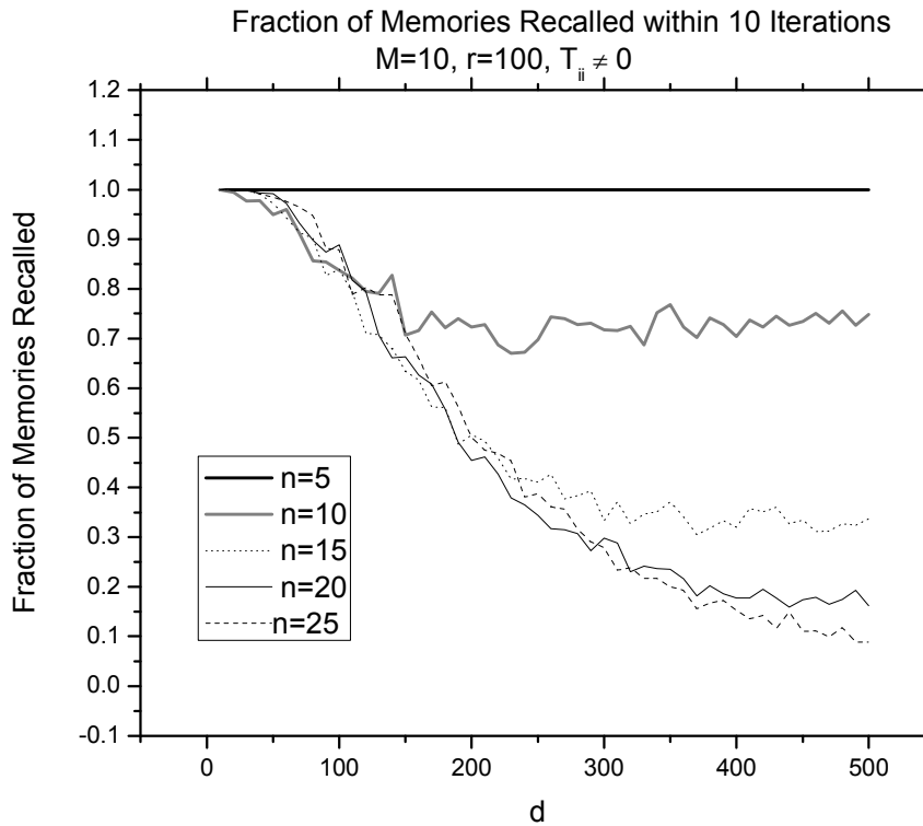
Fig. 9.7 – Fraction of Memories Recalled to Either a Spurious or Converged State within 10 Iterations as a Function of Vector Length ( d ) and Number of Memories Encoded in Network ( n )
