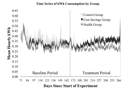
*Fig. S2* Time series of hourly community consumption. During the baseline period, the mean hourly kWh consumption is overlapping for all three groups. After treatment begins, the consumption diverges. Treatment effects are identified by difference-in-differences before-after-control-impact design.
