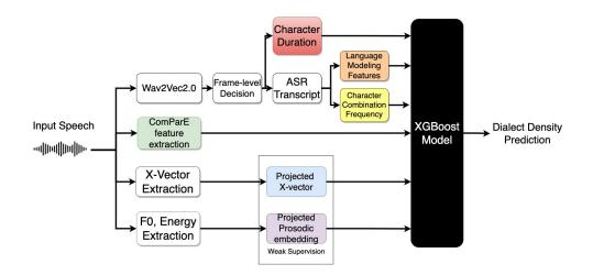
Figure 3.2: Overview of the features used in the proposed dialect density estimation proposed framework.
