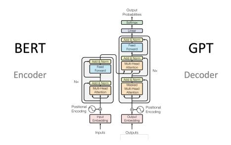
Figure 1.1: The transformer architecture consisting of the input layer, encoder stack, and decoder stack.
