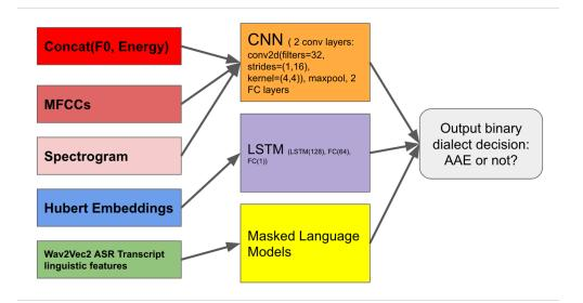
Figure 3.5: The feature set and backend models used in the proposed dialect identification scheme.
