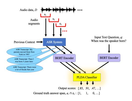
Figure 6.1: Overview of the proposed system. The long audio file, D is segmented into one minute segments,  $s_i$ . Each segment is then transcribed with ASR where the ASR system is prompted with previous context. Then both the ASR transcript from each segment and the text of an input query, q, are encoded with Sentence-BERT and scored for the likelihood that  $s_i$  answers q by the PLDA classifier. Last, the ground truth scores are used to evaluate performance.
