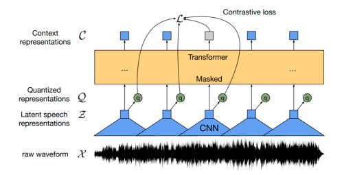
Figure 1.2: The Wav2Vec2 architecture, demonstrating how self-supervision is used to train the encoder layer to create a robust speech representation for downstream ASR or other tasks.
