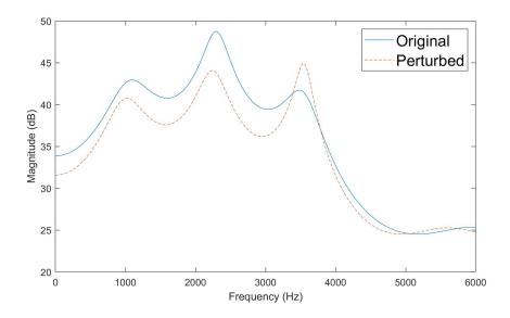
Figure 4.1: An example of the LPC spectra of a child in the UCLA JIBO kid's Database pronouncing the phoneme \AA\, and the result of perturbing it with LPC Augment. In the perturbed signal, the first two formant peaks have been shifted to the left, and the third has been shifted to the right.
