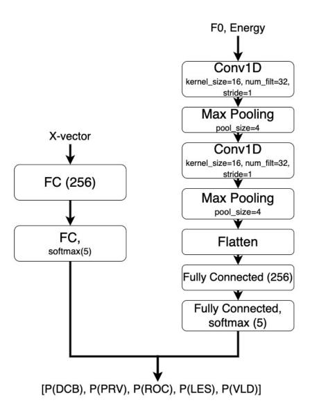
Figure 3.1: The architecture for the fully connected (FC) network used to project the X-vectors (left) and the CNN used to project the prosodic information (right). The inputs to the CNN are the pitch (F0) and three energy contours of the utterance. The output of both networks is a vector whose elements represent the probability of the speaker belonging to each of the cities used from the CORAAL database.
