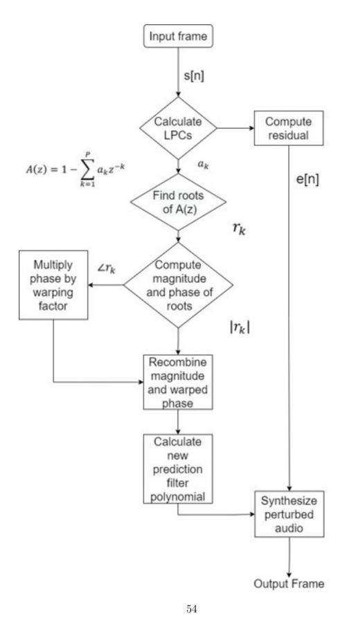
Figure 4.2: Diagram of the LPC Augment Algorithm
