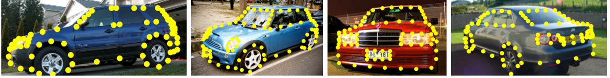
Figure 3.5: The landmark annotations for typical images. Yellow dots are the annotated landmark locations. Please refer to Section 3.3.3 for landmark selection criteria.
