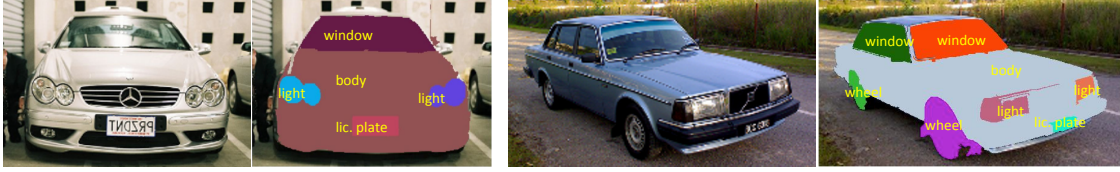
Figure 3.1: The goal of car parsing is to detect the locations of semantic parts and to perform object part segmentation. The inputs (left) are images of a car taken from different viewpoints. The outputs (right) are the locations of the car parts – the wheels, lights, windows, license plates and bodies – so that each pixel within the car is assigned to a part.
