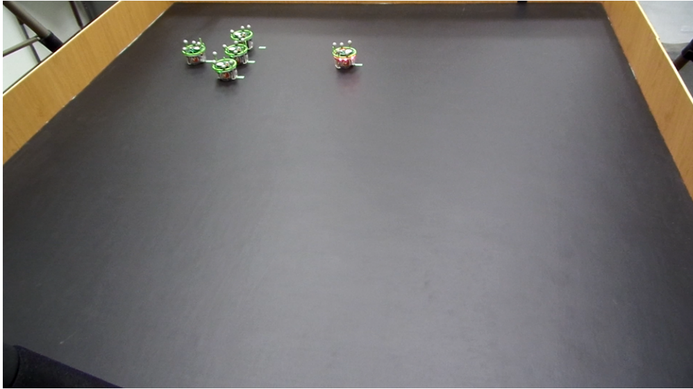
Figure 7.9: Robot experiment setup with five e-puck robots. Each robot has a unique configuration of infrared reflecting markers (green rings with silver spheres) tracked by a motion capturing system with four Bonita 10 Vicon cameras. The robots are at their initial position (see Fig. C.2 in Appendix C).
