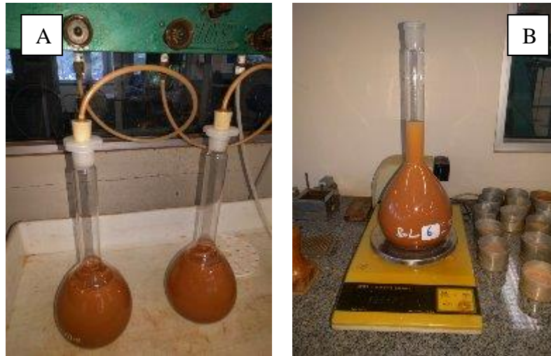
Figure 4.14. 4.13A and 4.13B. Fig. 4.13A illustrates the air being removed from the mixed material with a vacuum pump. Fig. 4.13B illustrates mixed material being weighed to compute the particle soil density
