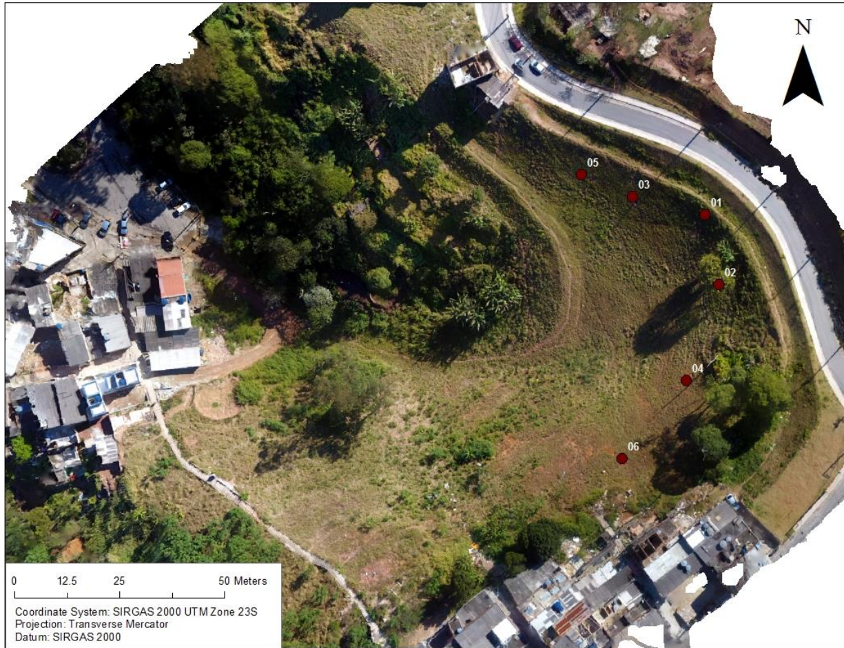
Figure 4.4. Disturbed site. Red dots indicate locations at which soil was collected and hydraulic conductivity test was conducted in situ. (Source: Author)
