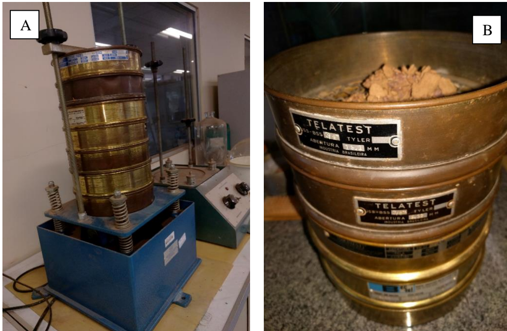
Figure 4.12. 4. 11A and 4.11B. Fig. 4.11A illustrates the machine with the sieves to sift the soil grain and separate them based on their grain size. Fig. 4.11B illustrates the coarse soil on top of the sieves ready to be placed in the machine.
