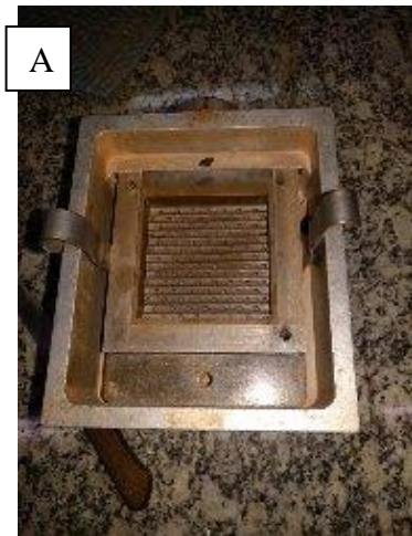
Figure 4.17. Fig. 4.16A and 4.16B. Fig. 4.16A shows location in which the molded soil sample was placed to do the shear stress test. Fig. 4.16B illustrates the shear stress test machine used in this study.
