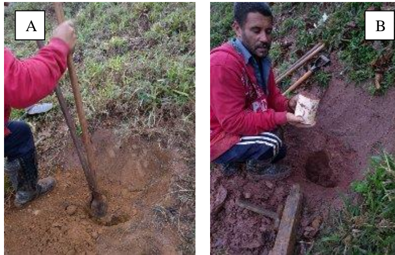
Figure 4.15. 4.14A and 4.14B. Fig. 4.14A illustrates the use of the hole digger to take the soil sample using PVC pipe. Fig. 4.14B illustrates soil collected with the PVC pipe.
