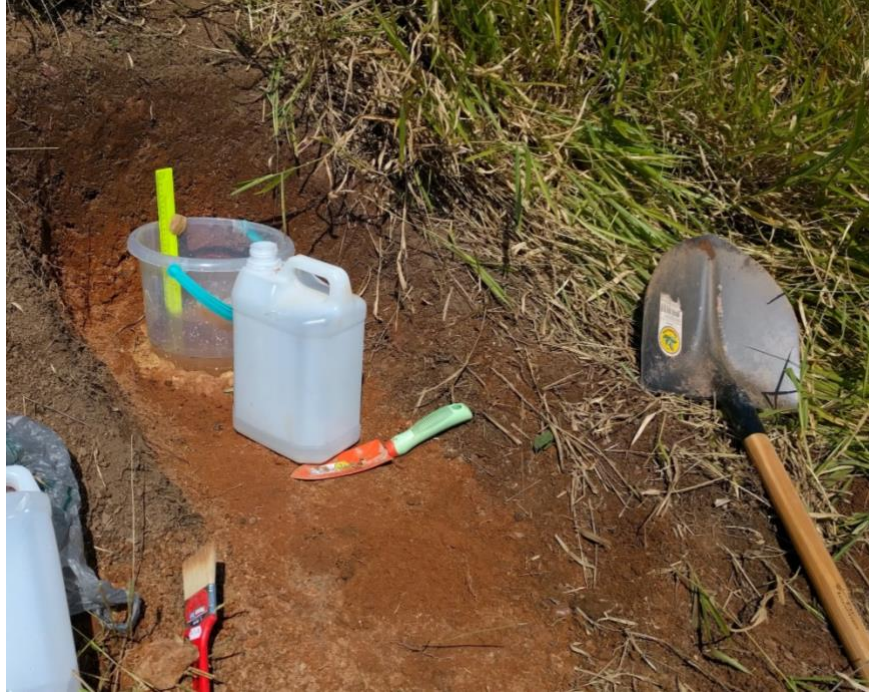
Figure 4.8. One of the sites in which the field-saturated hydraulic conductivity was measured. The area was first cleared with the shovel and the paintbrush to place the bottomless bucket. Between the outer part of the bucket and the soil, clay was spread to avoid lateral water leakage. Water was placed inside the bucket and the time that the water took to infiltrate the soil was measured.
