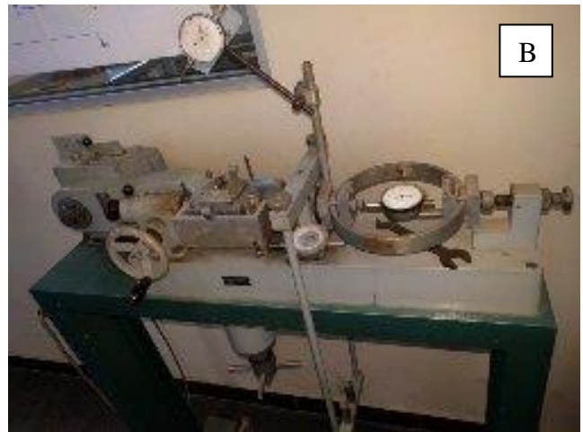
Figure 4.17. Fig. 4.16A and 4.16B. Fig. 4.16A shows location in which the molded soil sample was placed to do the shear stress test. Fig. 4.16B illustrates the shear stress test machine used in this study.
