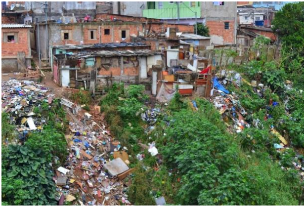
Figure 2.9. 2.9A and 2.9B. Fig. 2.9A illustrates slope with garbage and construction material mixed with soil in landslide risk area in Sao Paulo (Source: Goto, 2012). Fig. 2.9B is detailed photo of the material mixed with soil (Source: Goto, 2012)
