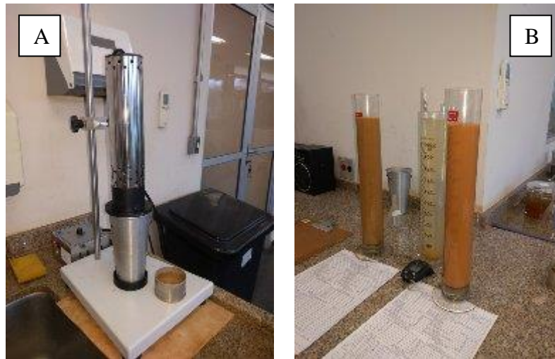
Figure 4.13. 4.12A and 4.12B. Fig. 4.12A illustrates the soil dispenser machine that mixed the dry sample soil, sodium hexametaphosphate, and distilled water. Fig. 4.12B illustrates mixed material (muddy color) in the graduated cylinder to measure the density and temperature over 24h.
