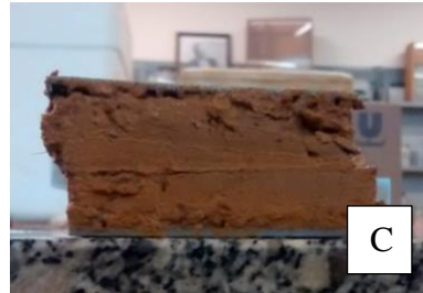
Figure 4.16. 4.15A, 4.15B, and 4.15C. Fig. 4.15A illustrates soil being molded inside the PVC pipe. Fig. 15B soil molded and ready to be used in the shear stress test. Fig. 4.15C shows the sample after its rupture.
