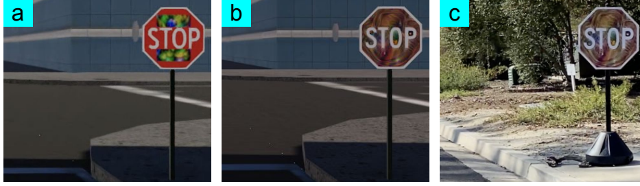
Figure 7.4: Reproduced semantic AD AI attacks on STOP sign hiding: (a) RP2 [157] in simulator, (b) SS [120] in simulator, and (c) SS [120] in physical world.
