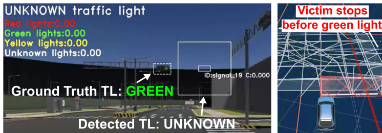
Figure 4.4: Snapshot of attacking the green light detection. The TL detector failed to detect any light in the ROI, causing the victim to stop at the stop line despite the light is green.
