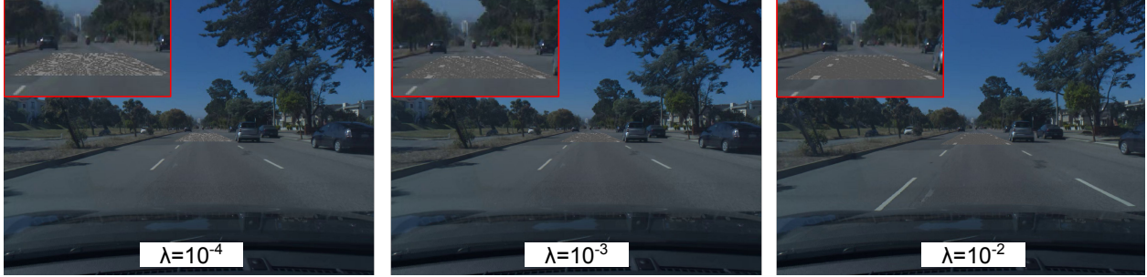
Figure 4.10: Driver’s view at 2.5 sec (average driver reaction time to road hazards [12]) before our attack succeeds under different stealthiness levels in local road scenarios. Inset figures are the zoomed-in views of the malicious road patches.
