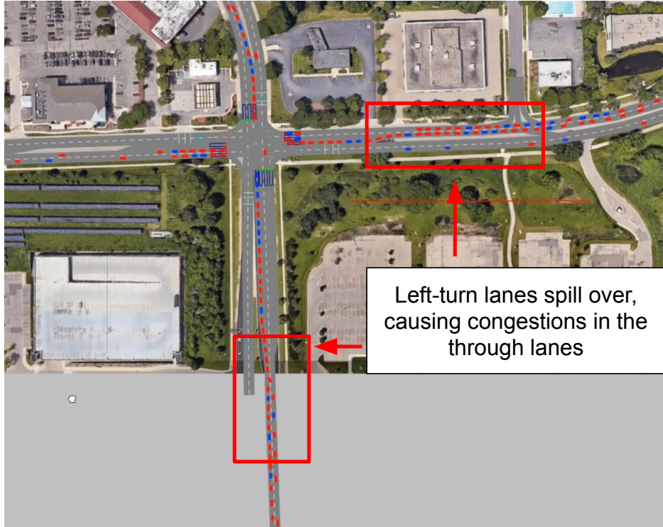
Figure 6.3: A Vissim snapshot of the traffic congestions caused by our reproduced attacks.
