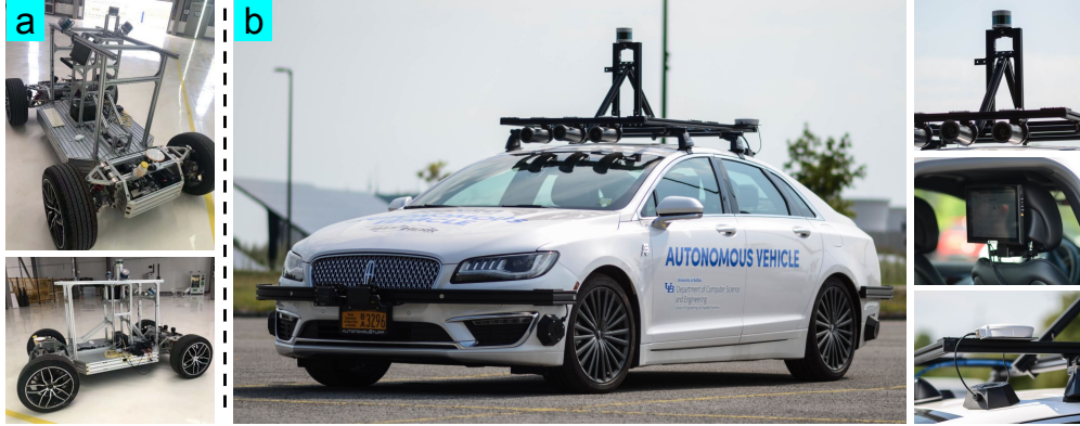
Figure 7.3: AD vehicles for the system-driven evaluation platform: (a) A real-vehicle sized chassis with L4 AD sensors and closed-loop control; (b) An L4 AD vehicle built upon Lincoln MKZ. Both are equipped with L4 AD-grade sensors such as LiDARs, cameras, RADARs, GPS, and IMU.
