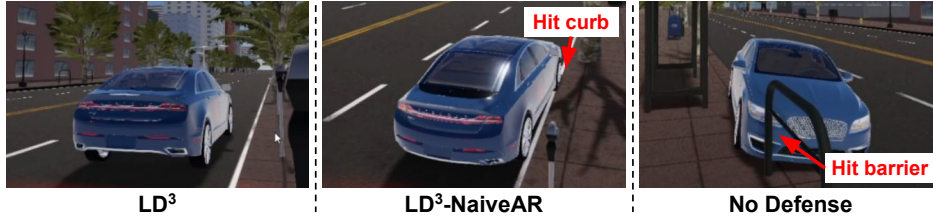
Figure 5.9: Simulation snapshots of the vehicle stopping locations under the 3 defense settings in SF-Straight.
