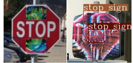
Figure 4.12: Stop sign hiding and appearing attacks [420].
