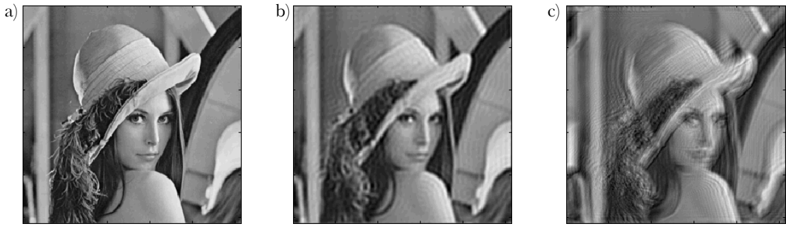
Figure 1.10: (a) An image from an optical system with enough resolution to see all of the features; (b) The image from an optical system with a wavelength that is 3 times as long; (c) The image from an optical system with original wavelength in the presence of aberrations.
