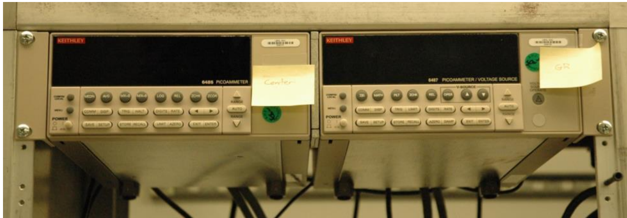
Figure B.11. Photograph of Keithley 6485 (left) and 6487 (right) picoammeters used for precision current measurement.
