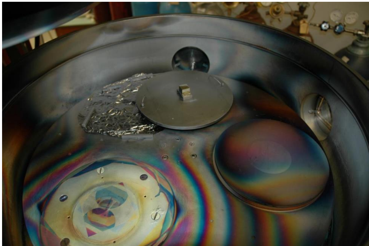
Figure A.9. Photograph of the inside of the main chamber of the MRC sputtering system. A crystal can be seen upper center on the rotation stage under the Ge target.
