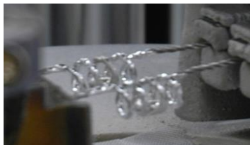
Figure A.12. Photograph of tungsten filaments pre-loaded with aluminum.
