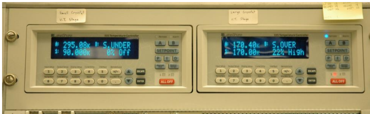
Figure B.12. Photograph of LakeShore 335 temperature controllers used for temperature readout and heater control of variable-temperature cryostat stages.
