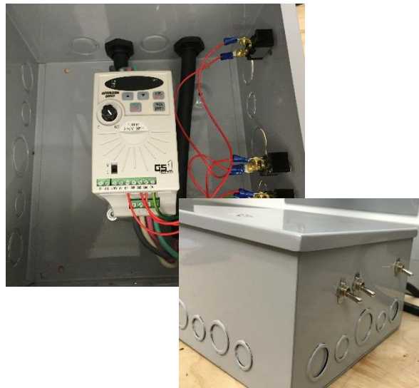
Figure 2-24: Motor control wiring schematic (left). Motor controller housing, and control switches (right).
