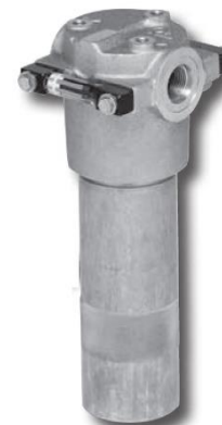
Figure 2-7: Donaldson HPK02 filter housing is compatible with DT Synteq filters, has a maximum working pressure of 2000 psi and a burst pressure of 4500 psi. It accepts flow rates up to 20 gpm [41].
