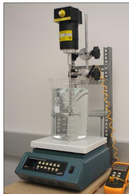
Figure 2-1: Fluid blending station utilized in this work, capable of heating and blending fluids in batches of up to 2 gallons.
