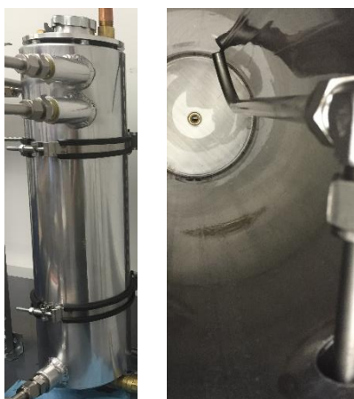
Figure 2-10: 2.125 gal. capacity oil reservoir with 6 in internal diameter provides sufficient capacity to extract ten 500 mL samples (left). The return line was plumbed to ensure return flow remains submerged (right)
