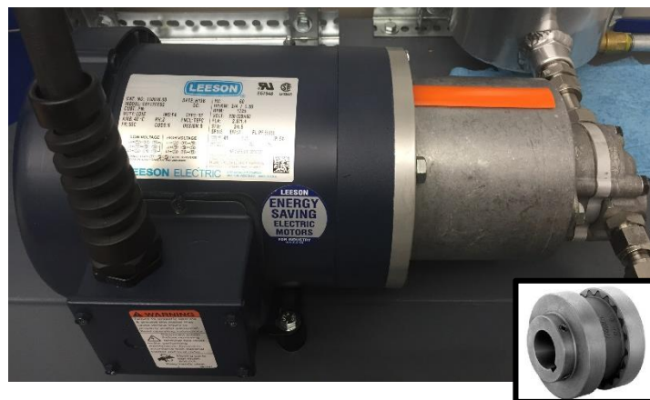
Figure 2-16: A \frac{3}{4} hp 3-phase 208V motor powers a 0.21 \text{ ci/rev} gear pump. The motor is coupled to the pump by a flexible coupling (insert) housed inside an aluminum bell housing. The flexible coupling allows for parallel and angular misalignments while absorbing both linear and torsional vibrations and shocks [51].
