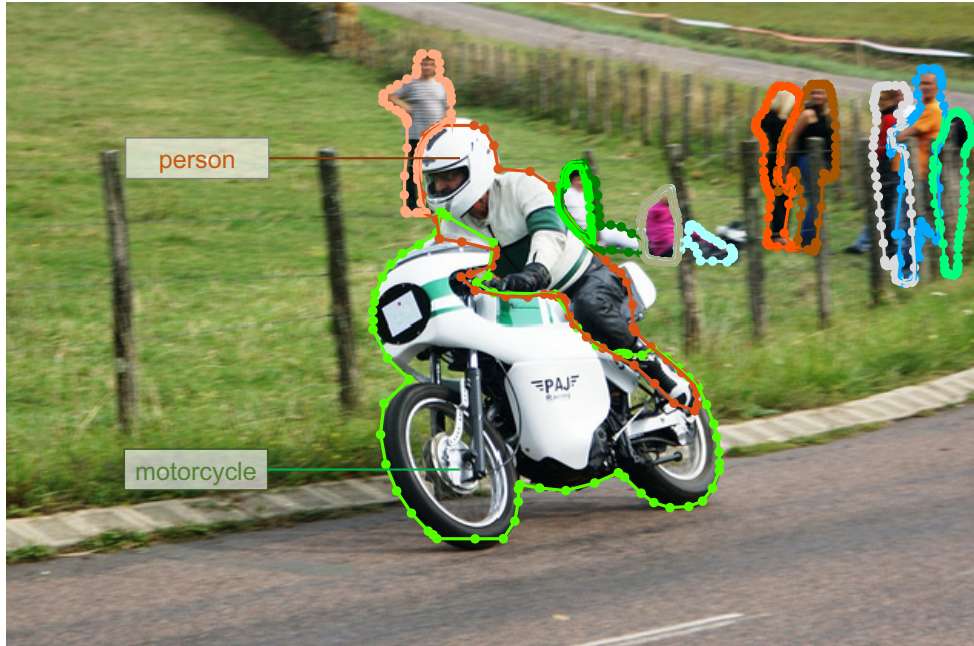
Figure 5.1: We present a model of instance segmentation which predicts the boundaries of each object in the form of a polygon. This treats instance segmentation as a regression problem and allows for end-to-end differentiability of predictions. At the same time, our model requires no sacrifices in terms of resulting segmentation quality nor introduces additional supervision requirements compared algorithms which directly predict masks.
