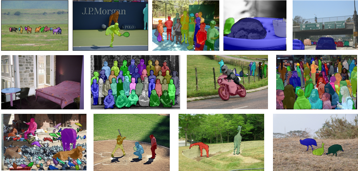
Figure 5.4: BoundaryFormer is able to predict high quality instance segmentations over the MS-COCO dataset: Predicted boundary points are shown in black. The resulting rasterized mask is overlaid onto the instance in color.
