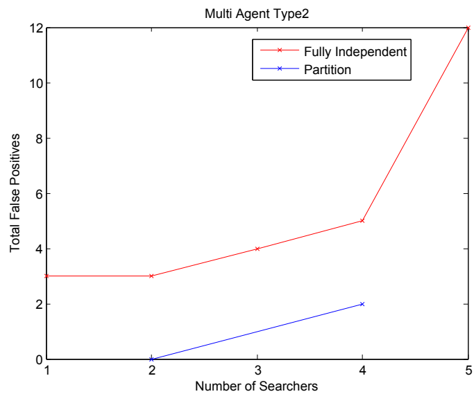
Figure 5.14: Total number of false positives over 100 runs for varying amounts of searchers. Patrolling was only tested with 2 and 4 searchers.
