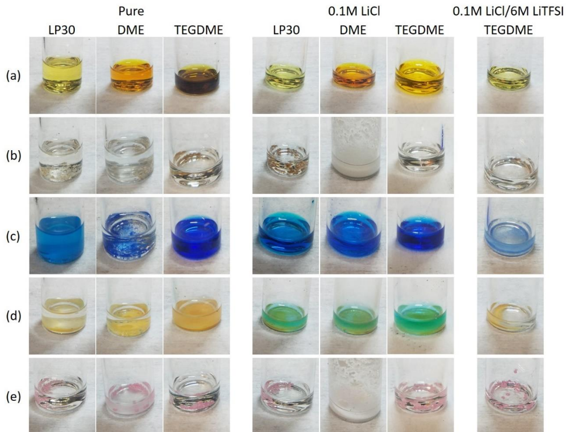
Figure 2.1 Transition metal chloride dissolution test in each solvent: (a) \text{FeCl}_3 , (b) \text{FeCl}_2 , (c) \text{CoCl}_2 , (d) \text{NiCl}_2 , (e) \text{MnCl}_2 in pure LP30 (EC:DME = 1:1 with 1M \text{LiPF}_6 ), pure DME, pure TEGDME, 0.1M LiCl LP30, 0.1M LiCl DME, 0.1M LiCl TEGDME, and 0.1M LiCl/6M LiTFSI TEGDME.
