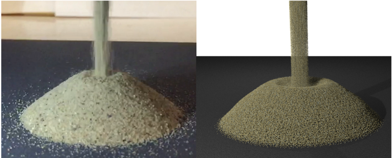
Figure 4.10: Sand is poured from a spout into a pile in a lab (left) and with our method (right).
