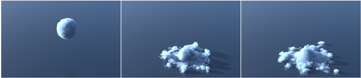
Figure 2.12: Our approach works naturally with the material point method simulations from [SSC13]. Here we demonstrate with a snowball that drops to the ground and fractures. Notably, we provide a new treatment of particle position updates that naturally prevents penetration in solid objects like the ground.
