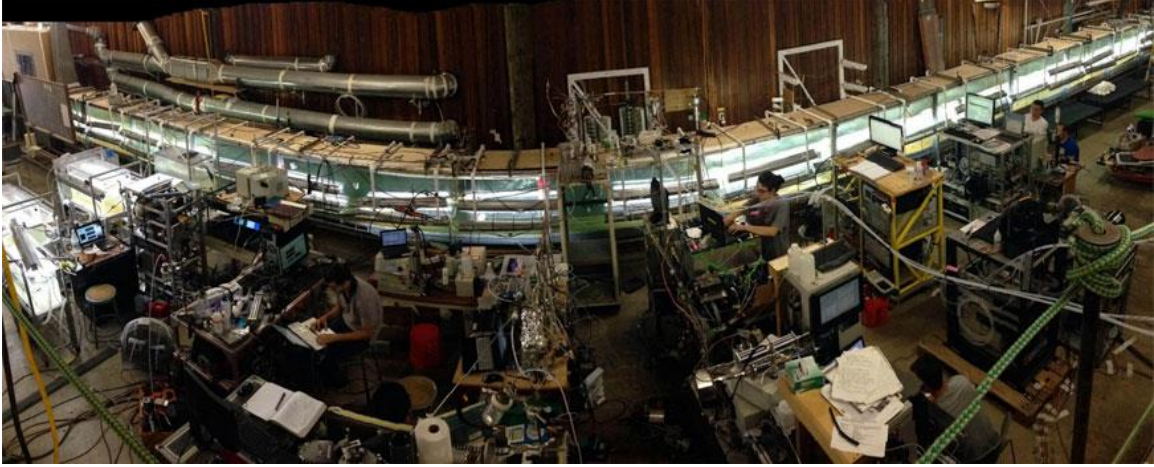
Figure 1.5: Image of the 30-meter-long wavechannel used during the 2014 IMPACTS experiment in the Hydraulics Laboratory at Scripps Institution of Oceanography. The wavechannel was filled with filtered seawater and spiked with nutrients to produce a phytoplankton bloom. Aerosols were generated using a hydraulic paddle on the left end of the channel. A plank was used to mimic a beach upon which wave broke, producing SSA. Generated SSA were collected from a manifold for off-line and on-line analysis.
