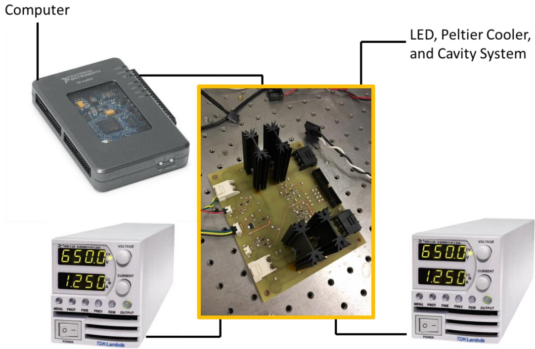
Figure 6.2: Schematic of the circuit board, power supplies, and MyRIO control. The computer interacts with the MyRIO through Labview to control the power supply of the LED and Peltier cooler and to give temperature readout of the thermocouples.
