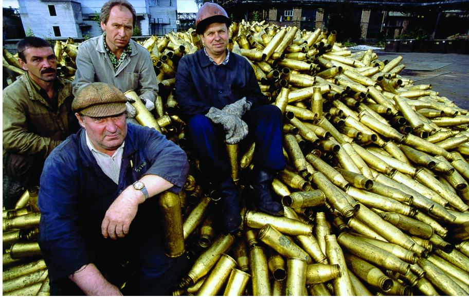
Figure 3.10: Photo showing the the Russian Navy shells re-purposed for the CMS HCAL. From Ref. [38]
