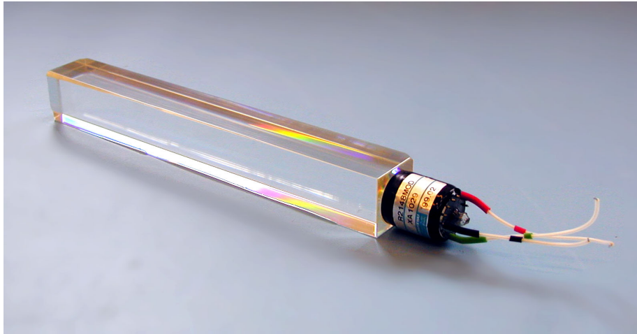
Figure 3.8: Photo of ECAL crystal with photodiode. From Ref. [36]
