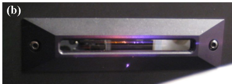
Figure 2.7 (a) Photograph of SLM (front), with dashed line around entrance polarizer. (b) Close up of entrance polarizer, showing faint back reflection of broadband laser spectrum.
