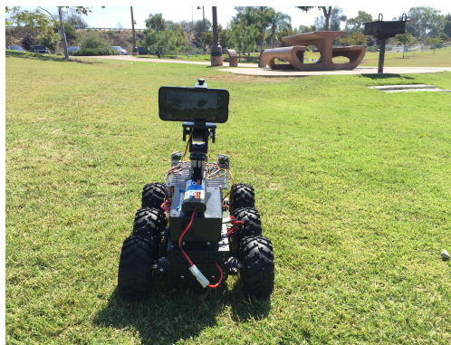
Figure 4.1: A six-wheel Android-based ground robot (ABR) used for terrain classification experiments.
