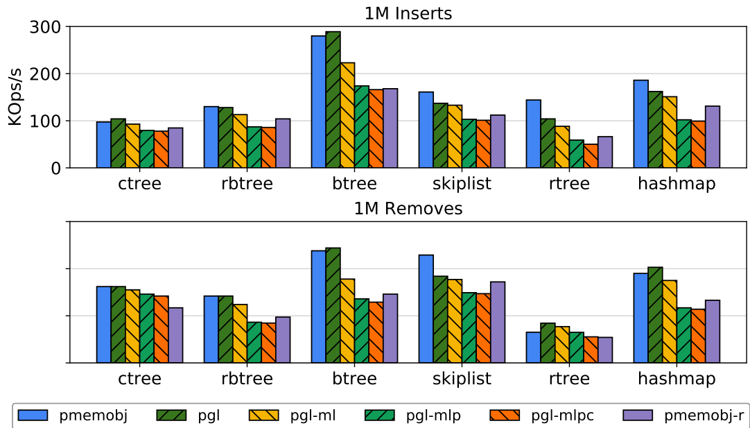
Figure 3.5: Key-value store performance - Each transaction either inserts or removes one key-value pair from the data store.
