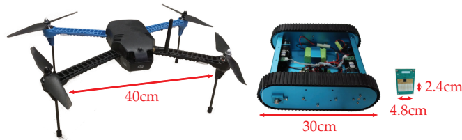
Figure 2.19: The actual size comparison of a drone, a robot car and our 60GHz array prototype. The array (16×8) is compact and both TX and RX can be mounted on a single mobile device.
