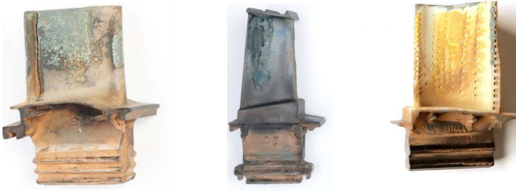
Figure 1. First stage turbine blade degradation from particulate ingestion [13].
