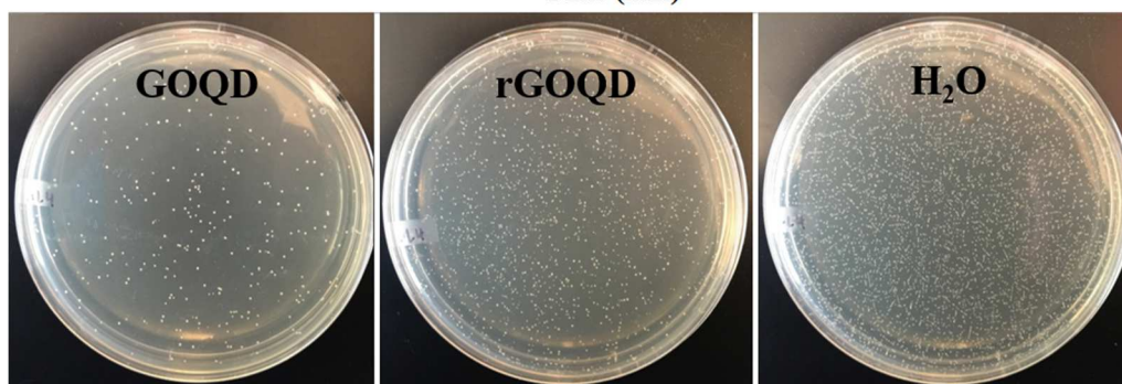
Figure 8. Summary of colony-forming units counted from agar plates inoculated by bacterial cells at increasing incubation time with GOQD, rGOQD, and pure water as a control with photographs of the plates inoculated by bacteria after 3 minutes of incubation.
