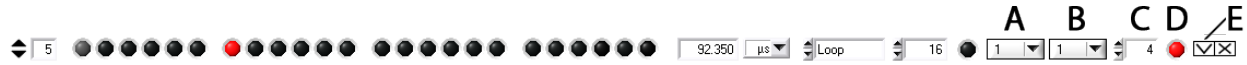
Figure 4.6: The initial state of a phase cycled instruction when phase cycling is turned on. The instruction to display is selected using the pulldown labeled A . B is used to select the phase cycle along which this instruction should vary. C sets the number of steps in the phase cycle (and updates all other instructions varying along the same cycle). D toggles phase cycling on and off, and E is used to collapse or expand the full phase cycle view.
