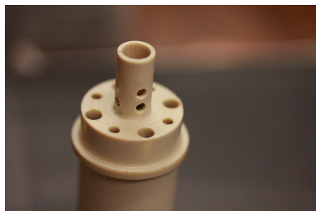
Figure 3.8: Vents are placed in the bottom of the probe head to allow air displaced by the falling sample tube to escape rapidly; without these, air is compressed below the NMR tube, slowing or stopping entirely its descent before it reaches the measurement region.
