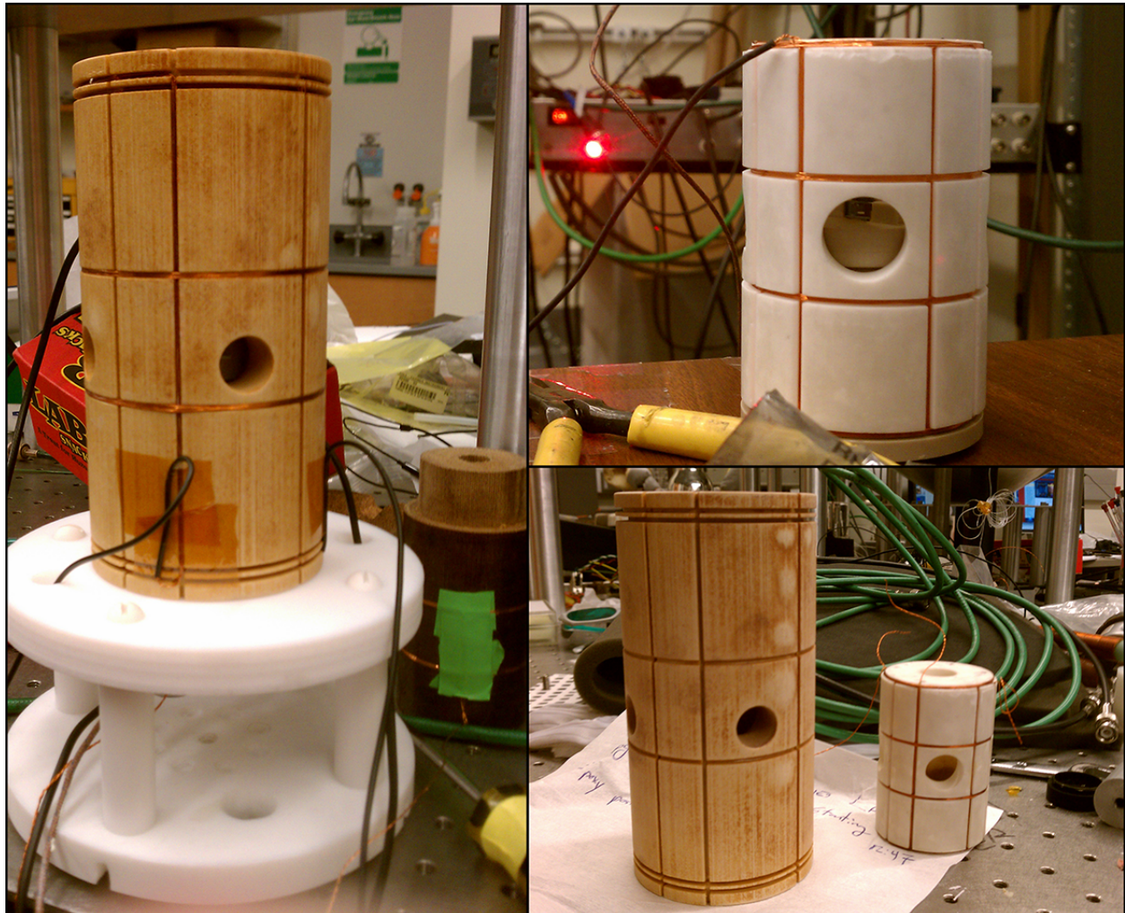
Figure 3.10: Photographs of the new pulse coil assembly (left), old pulse coil assembly (top right) and a comparison between the new and old substrates (bottom right).
