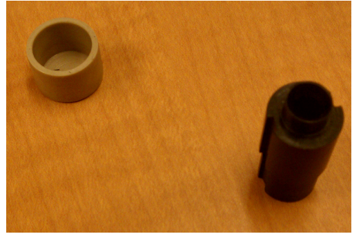
Figure 3.5: An older version of the probe head, with a flat-bottomed cap.
