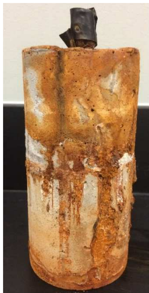
Figure 8.15 0% SHC at different corrosion stage. (a) during accelerated corrosion test; (b) one month under non-accelerated corrosion
