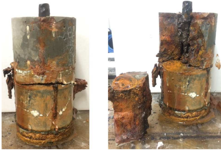
Figure 8.17 0% Mortar at different corrosion stage. (a) during accelerated corrosion test; (b) one month under non-accelerated corrosion
