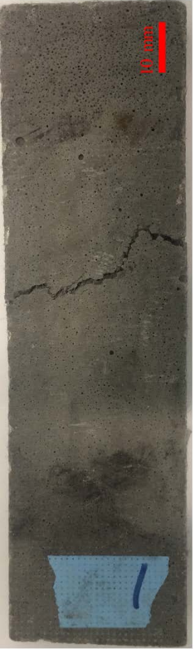
Figure 6.19 Image reconstructions of coupon specimen N2 with a localized crack
