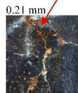
Figure 8.16 5% MSC at different corrosion stage. (a) during accelerated corrosion test; (b) one month under non-accelerated corrosion
