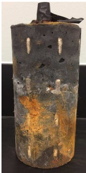
Figure 8.16 5% MSC at different corrosion stage. (a) during accelerated corrosion test; (b) one month under non-accelerated corrosion
