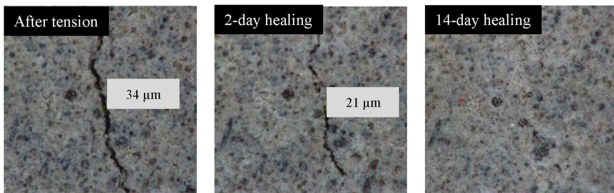
Figure 5.27 Optical microscopy and SEM images of self-healing phenomenon in SHC
