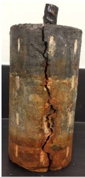
Figure 8.18 5% Mortar at different corrosion stage. (a) during accelerated corrosion test; (b) one month under non-accelerated corrosion
