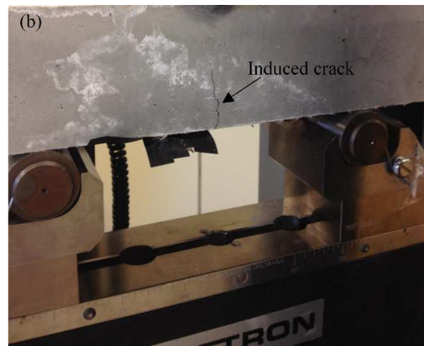
Figure 6.14 Beam specimen under four-point bending test: (a) test setup and dimension; (b) crack in the mid-span of the beam
