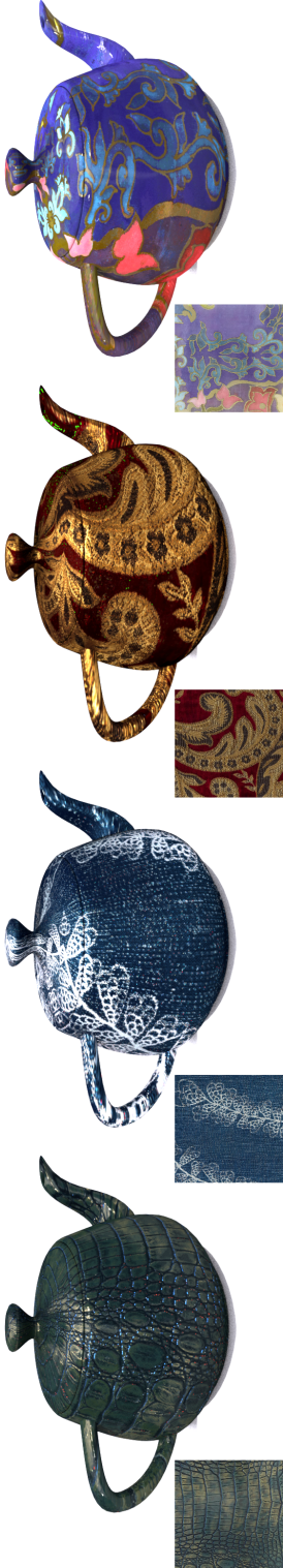
Figure 1.1: Four materials captured using my method and rendered with Mitsuba. Objects are illuminated by the Uffizi environment map (courtesy of the USC Vision & Graphics Lab) along with two point light sources. The left two materials were captured with one camera, and the two on the right were captured with two cameras. From left to right: green faux leather, blue damask fabric, red velvet lamé, and wrapping paper. Inset image shows the average color per pixel as described in section 3.2.
