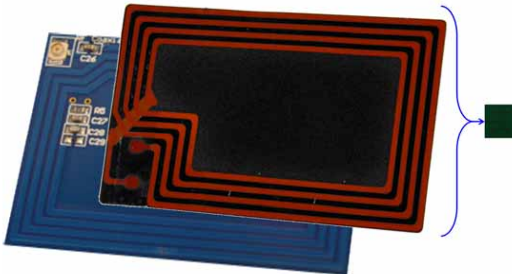
Fig. 1.3 The back and front sides of an NFC tag which is 6 \text{ cm} \times 4 \text{ cm} versus a 60 GHz 2 \times 2 microstrip patch antenna array with an area of 6.6 \text{ mm} \times 6 \text{ mm} .
