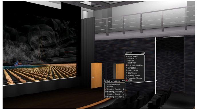
Figure 4: The video playback plugin embedded into a virtual theater VR application. Users can navigate into the theater and watch high resolution videos. The virtual theater application renders 201,688 polygons.
