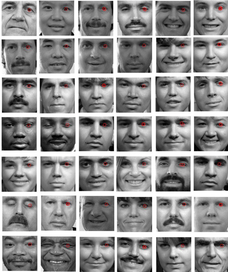
Figure III.8: Successful detection and localization of left eye. The detections are marked by red circles.
