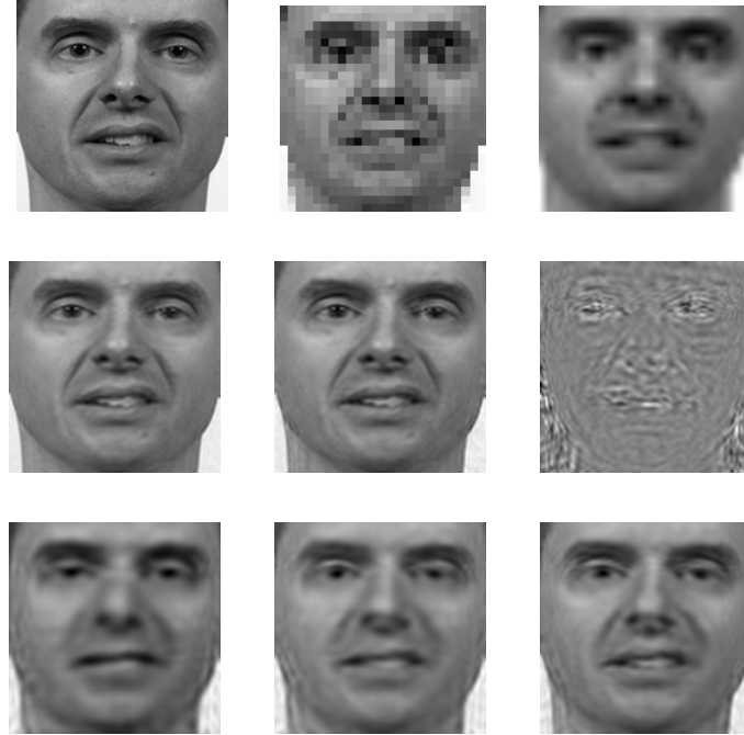
Figure VI.17: Top (left to right): original image, LR input and bilinear interpolation; middle: reconstruction results( \alpha = 0.99 ). From left to right: linear + RBF; linear only; and RBF only. Bottom: reconstruction results ( \alpha = 0.96, 0.97, 0.98 ).
