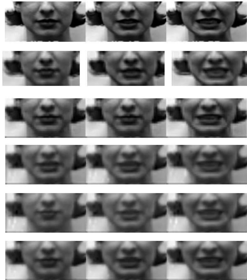
Figure VI.11: First row: the original HR images; second row: from the proposed inter-pixel interference elimination based algorithm; third row: from Borman's algorithm; fourth sixth rows: from different variant of the back-projection algorithm.
