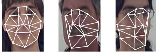
Figure V.8: Examples of the model face graph. The leftmost one is for the frontal view. The middle one is for the pose with 0^\circ tilt angle and -15^\circ pan angle. The rightmost one is for the pose with tilt angle 0^\circ and pan angle +15^\circ .
