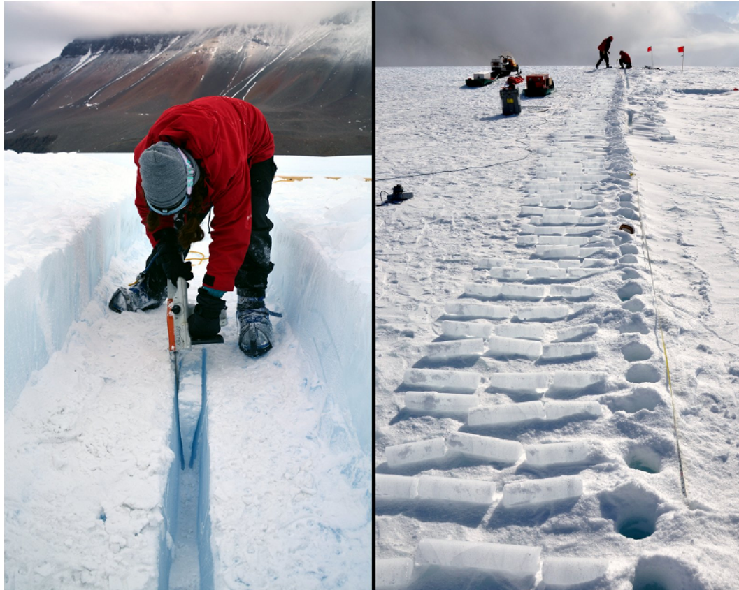
Figure 3.2: Impressions from sampling the horizontal ice core. (left) A. Palardy cutting a wedge of ice from the bottom of the trench for continuous analysis. (right) Sampling setup for discrete samples from 1 m depth. Some drilling holes are slightly offset to avoid cryoconite holes that could damage the cutters.
