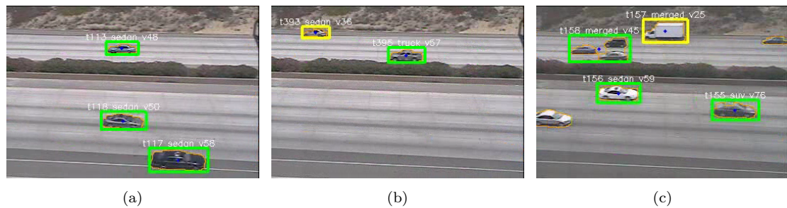
Figure 5.21: Highway I5 abnormalities. (a) Vehicle on shoulder during entrance. (b) Vehicle slows to exit in northbound direction on top of image. (c) Truck falsely identified as abnormal because detection centroid is high and appears to be on the side of the road.
