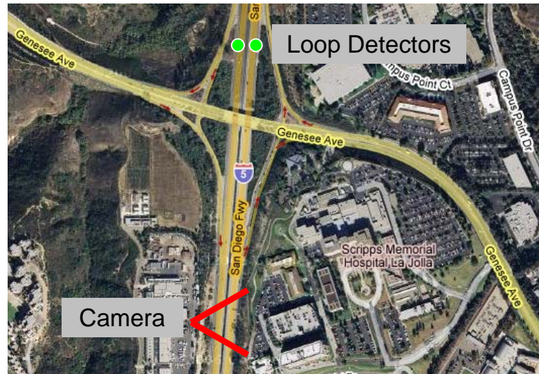
Figure 5.16: Camera and PeMS loop detector sensor configuration on opposite sides of the Genesee Ave. ramp.
