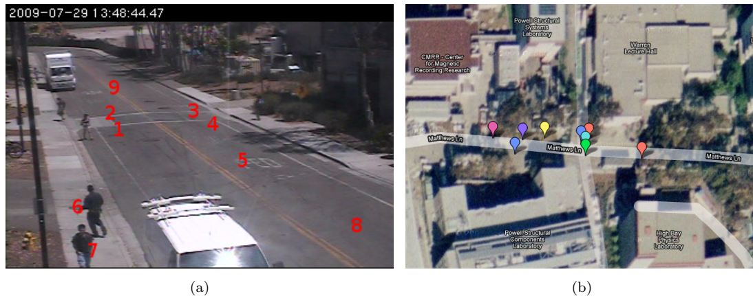
Figure 6.4: Geo-registration calibration with GPS coordinates obtained using an iPhone. (a) Image locations of ground plane calibration points. (b) Google maps satellite image with GPS location of calibration points.
