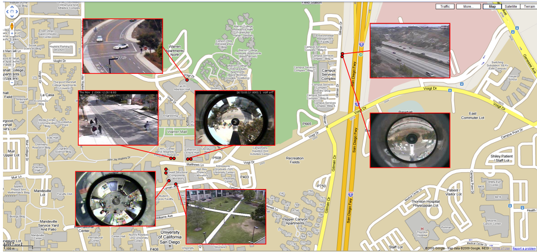
Figure 6.2: UCSD video network. A network of video cameras is situated around campus to provide coverage of different environments. Both rectilinear PTZ as well as omni-directional cameras are used to monitor highway vehicle traffic and the close interactions of people and vehicles on campus.
