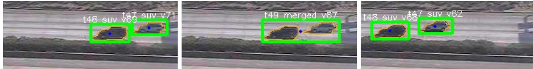
Figure 3.1: Occlusion causes initialization of new trajectories. When the occlusion is of short duration the tracking module is able to recover the correct trajectory labels.
