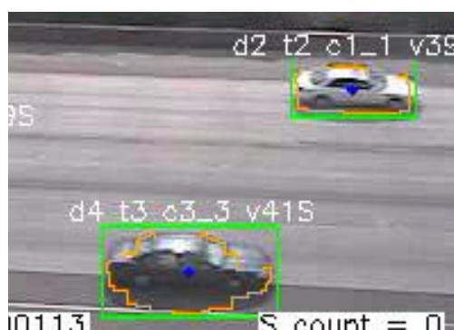
Figure 5.15: Object detection corrupted by shadows making a sedan appear as a SUV.
