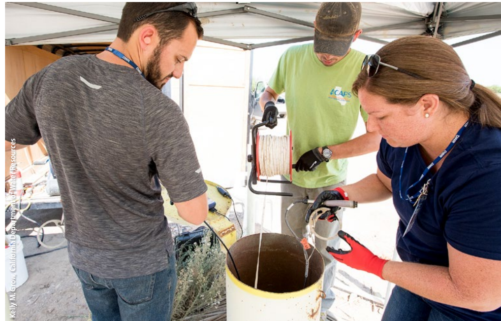
DWR staff members measure groundwater elevations using a handheld computer and electronic sounder at a well in Sutter County.
