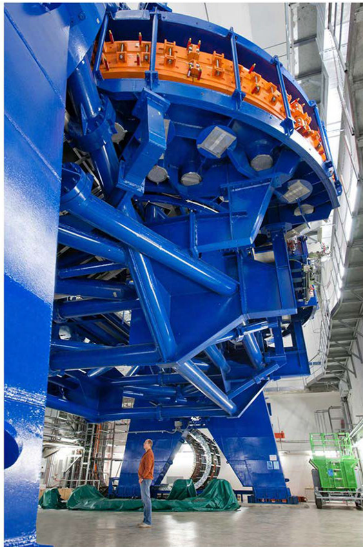
Photo of the first carbon gantry built in Heidelberg, Germany shows the size of the gantry relative to a person.
