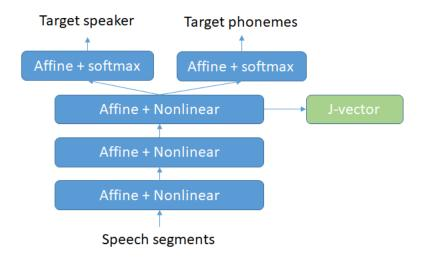
Figure 6.1. Structure of j-vector model
