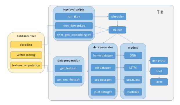
Figure 5.1. System Design of TIK
