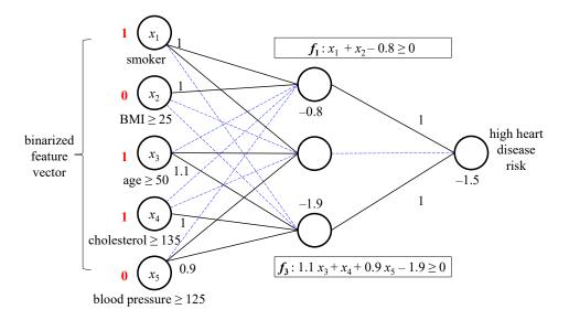
**Figure 3.1.** A toy example of the CT-Net architecture with hidden layer neurons as threshold logic functions and the output neuron implementing a conjunction.
