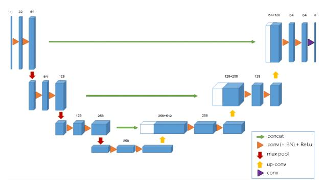
**Figure 6.1.** The 3D U-Net architecture. Activations are shown as blue cuboids whereas layers and other operations are displayed as arrows. The numbers above cuboids denote the channels of activations.
