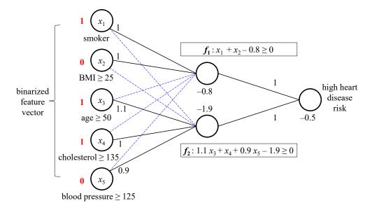
**Figure 2.1.** An example of the DT-Net architecture. Each hidden layer unit implements a threshold logic function, and the output unit implements a disjunction of these threshold functions. Explanations can be readily derived from the network to explain positive predictions.
