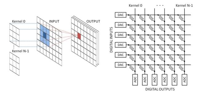
**Figure 5.2.** The ReRAM-based crossbar structure.
