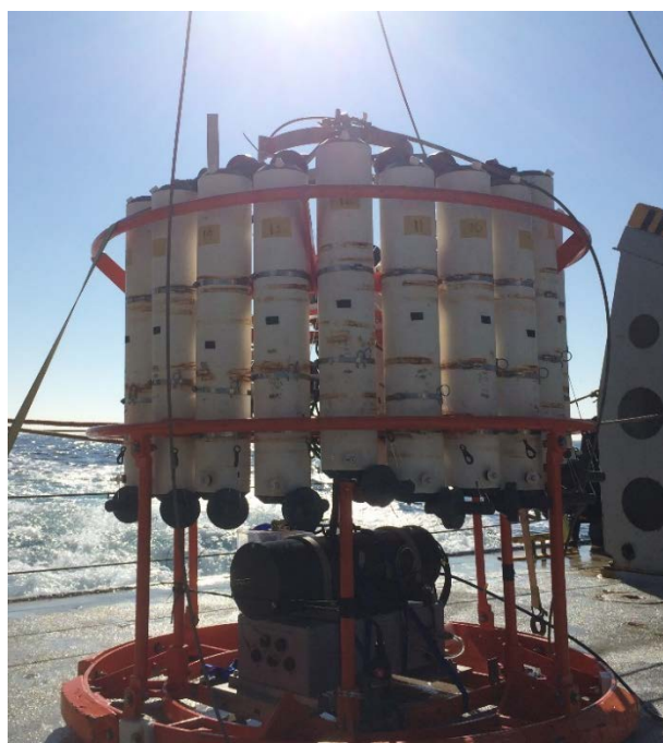
Figure 2.4. Micro-Rosette fastened to bottom of R/V Sproul's rosette frame, along with 16 Niskin bottles.
