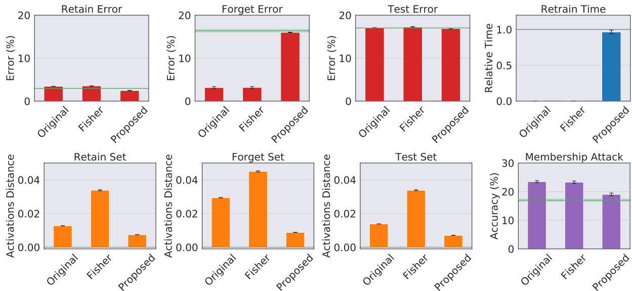
Figure 6.3: Read-out functions for different forgetting methods. We forget a subset of 10% of the training data through 10 equally-size sequential deletion requests using different forgetting methods, and show the value of the several readout functions for the resulting scrubbed models. Ideally, the value of the readout function should be the same as the value (denoted with the green area) obtained on a model retrained from scratch without those samples. Closer to the green area is better. (Original) denotes the trivial baseline where we do apply any forgetting procedure. (Fisher) Adds Fisher noise as as described in ([GAS19a]), (ML-Forgetting) The model obtained with our method after forgetting. In all cases, we observe that ML-Forgetting obtains a model that is indistinguishable from one trained from scratch without the data, whereas the other methods fail to do so. This is particularly the case for the Retrain Time readout functions, which exploits full knowledge of the weights and it is therefore more difficult to defend against.
