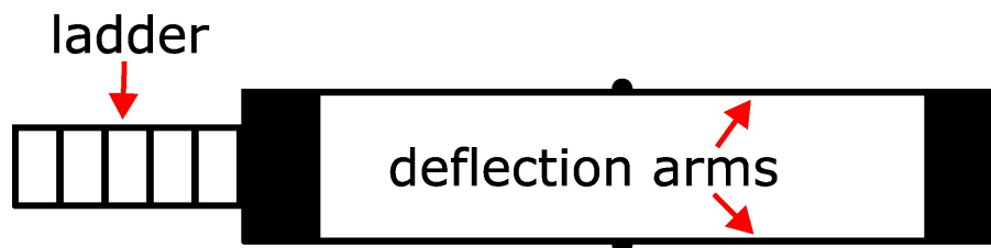
Figure 5.2: Schematic drawing of SU-8 deflection microtensiometer (not drawn to scale) [66]. Deflection arms are tracked optically to visualize the difference in surface pressure inside and outside the microtensiometer. Ladder is used to secure the position of the microtensiometer by feeding a wire through one of its holes.
