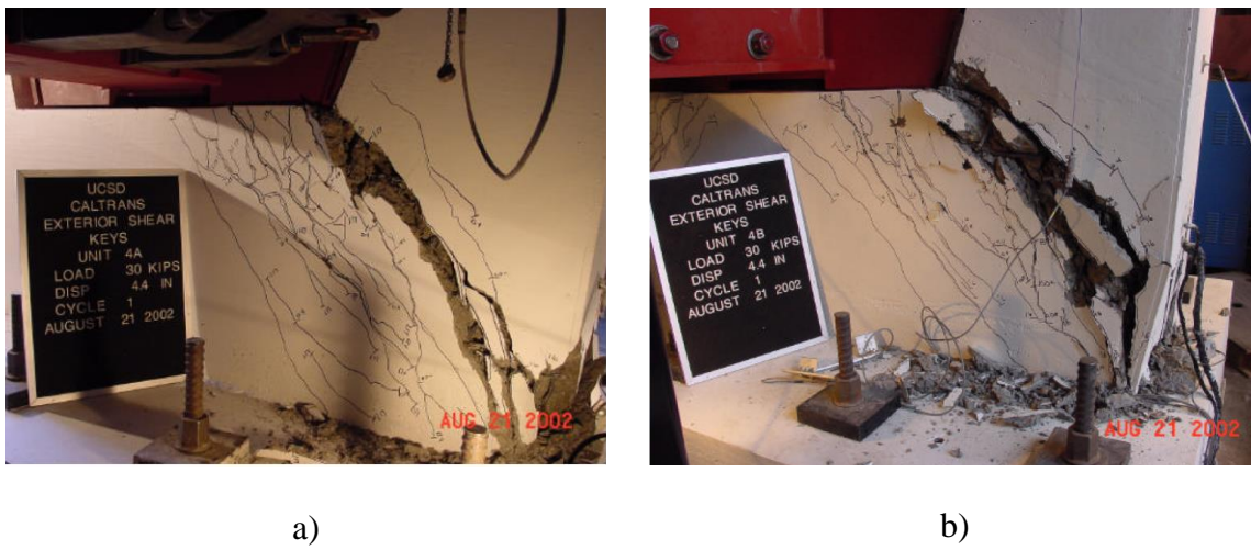
Figure 2.11 Condition of shear keys at the end of the test: a) shear key 4A; b) shear key 4B (from Borzozgadeh et al., 2006)
