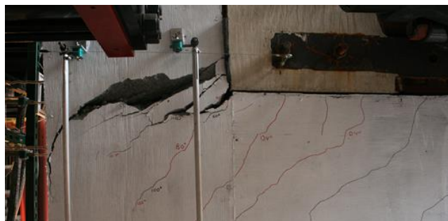
Figure 6.103 Sliding plane from the east face of shear key 10B
