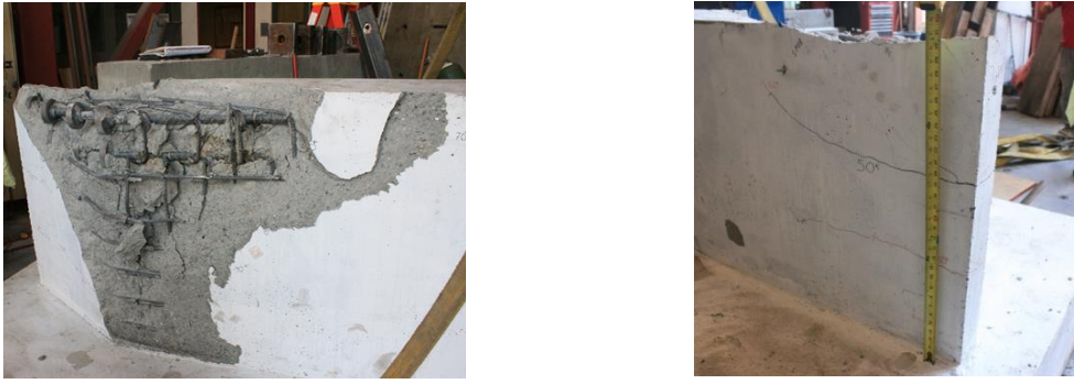
Figure 8.20 Shear plane from the northwest side (left) and from the southeast side (right) after removing shear key 12A
