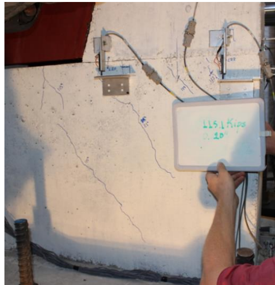
Figure 5.37 Diagonal cracks on the east side at 115 kips load in shear key 7B
