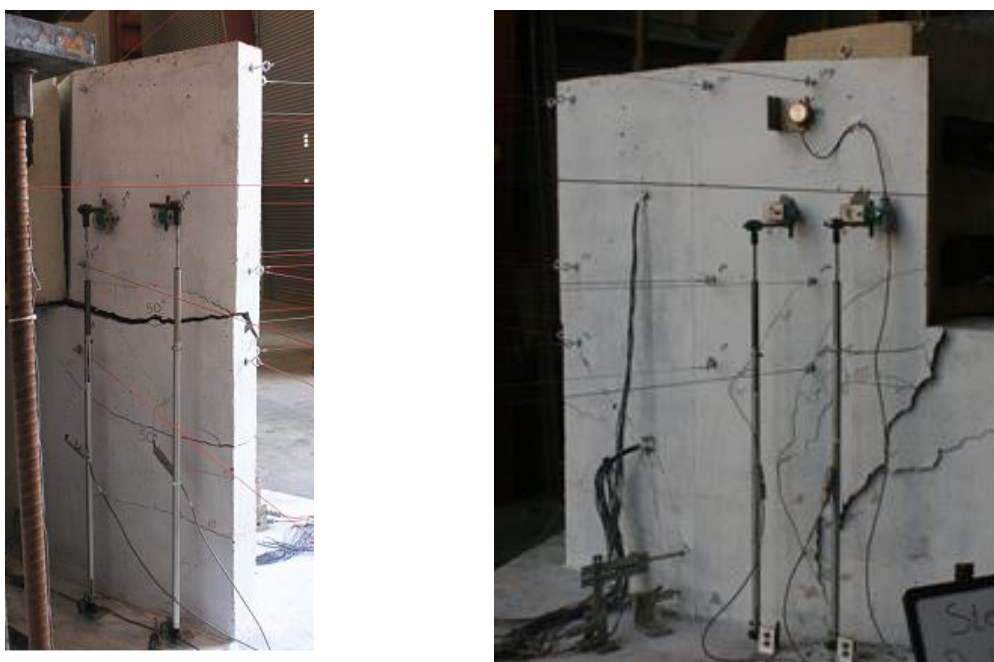
Figure 8.18 Cracks on the southeast side propagating to the northwest side (left) and cracks on the northwest side (right) of shear key 12A at a horizontal load of 70 kips
