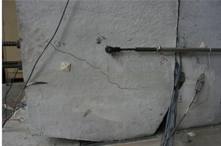
Figure 7.22 First crack (marked in red) observed on the west face of the shear key block in Test 4
