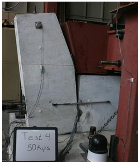
Figure 7.24 Displacement of shear key block at a horizontal load of 50 kips in Test 4
