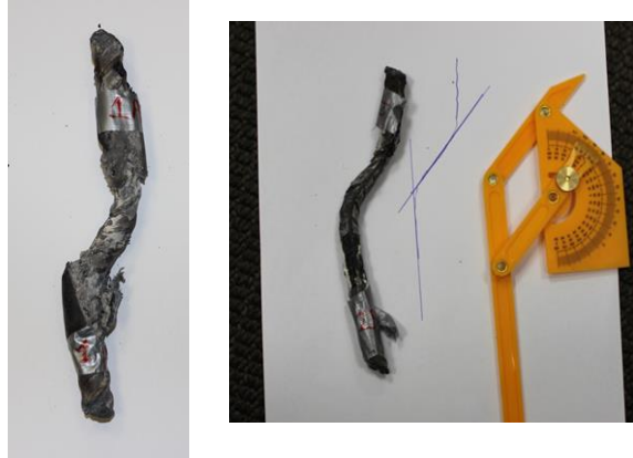
Figure 5.28 Extracted dowel bars from shear key 7A showing the angle of kink
