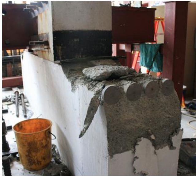
Figure 6.104 Sliding plane surface after removing shear key 10B
