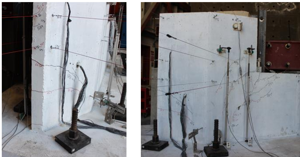
Figure 8.32 Cracks on the southeast side propagating to the northwest side (left) and cracks on the northwest side of shear key 12B at a horizontal load of 88 kips
