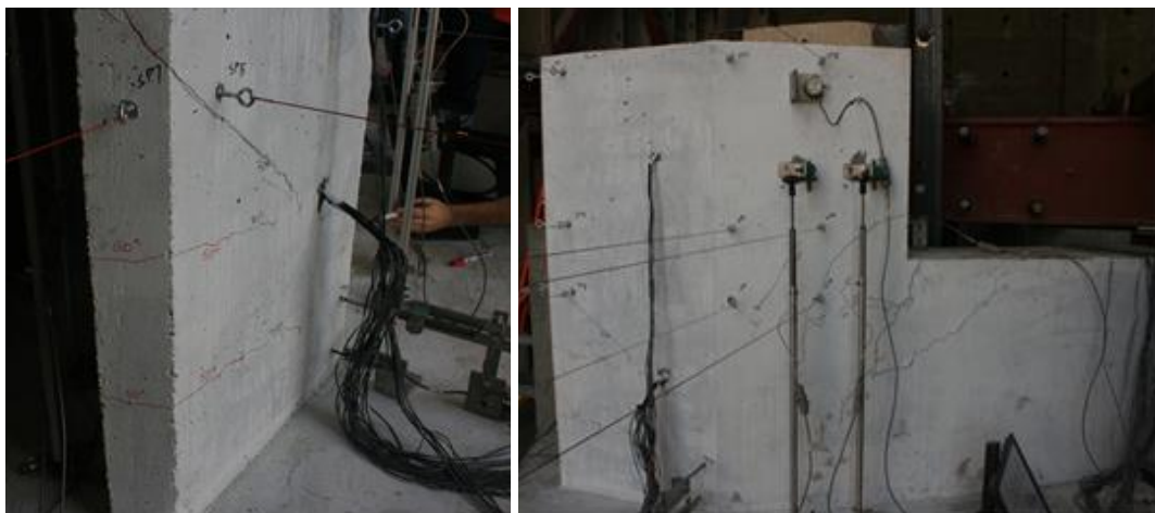
Figure 8.18 Cracks on the southeast side propagating to the northwest side (left) and cracks on the northwest side (right) of shear key 12A at a horizontal load of 70 kips
