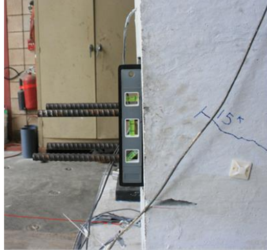
Figure 7.23 Monitoring the rotation of the outer plate in Test 4
