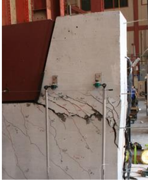
Figure 6.60 Sliding plane on the east face of shear key 9A
