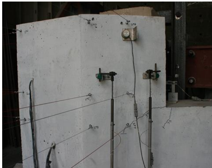
Figure 8.31 First cracks observed on the northwest side of shear key 12B
