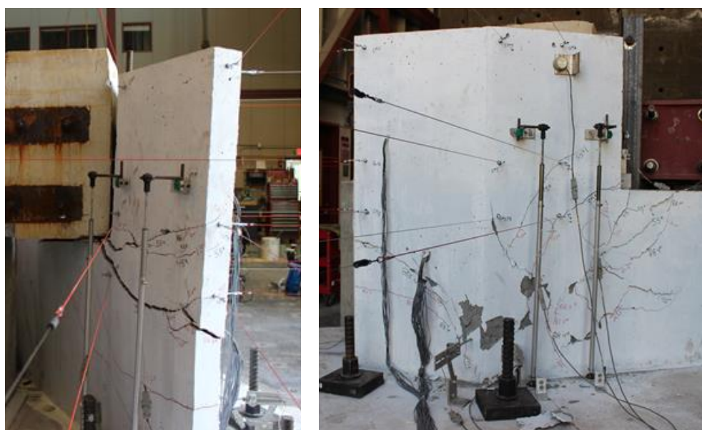
Figure 8.32 Cracks on the southeast side propagating to the northwest side (left) and cracks on the northwest side of shear key 12B at a horizontal load of 88 kips
