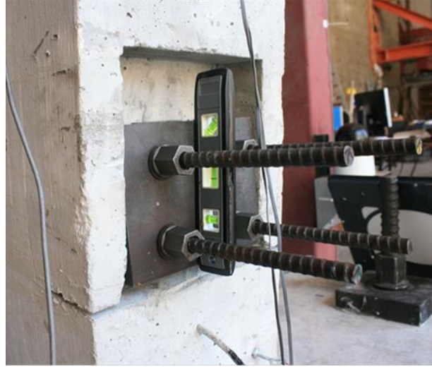
Figure 7.35 Monitoring the rotating plate in Test 5
