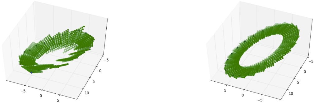
Figure 2.4: The chessboard poses for each turntable location are shown in the frame of the reference camera. On the left, the chessboard poses are determined by solvePnP. On the right, we refine these pose estimates using the plane equalization method described in Section 2.4.1. The refined board poses are significantly cleaner.
