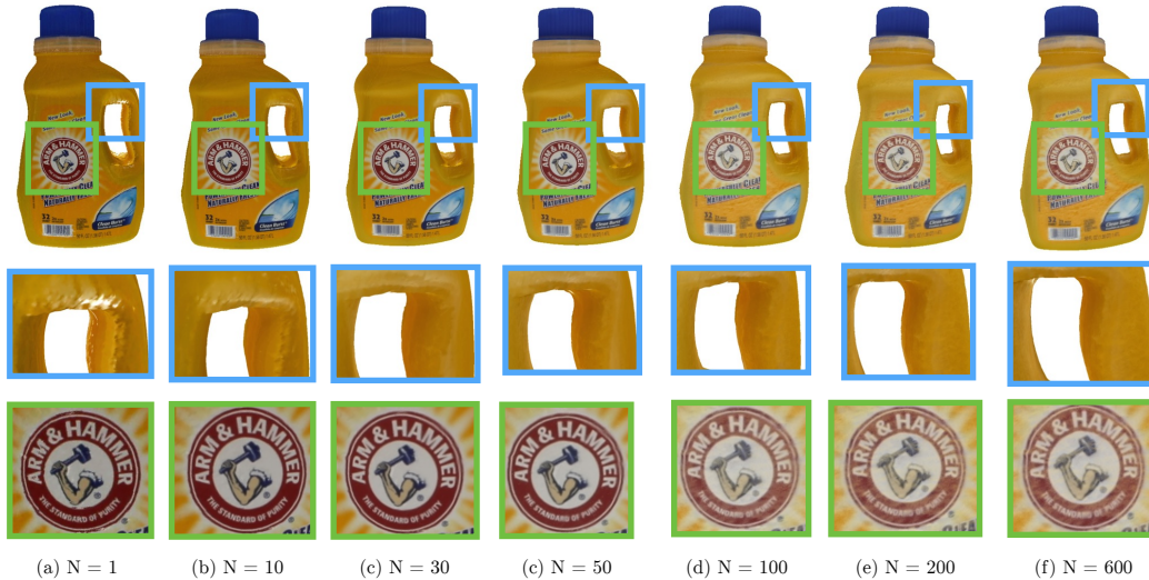
Figure 4.3: The effect of N = |V'(\mathbf{p}; t_{\mathbf{p}})| on the sharpness of textured regions and the smoothness of non-textured regions: smaller (larger) N yield sharper (faded) textures, but blotchy (smooth) non-textured regions. When N = 1 , we observe white regions on the detergent handle because these colors incorrectly bleed onto the white turntable background in the best viewing image; larger N rectify this problem.
