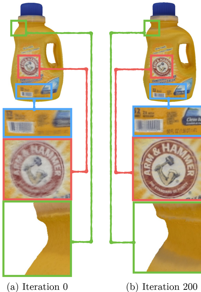
Figure 4.2: Mesh coloring (a), before, and (b), after, optimization using our implementation of the approach employed by Zhou et. al. 118 . Although this method improves texture coherence, the textures are still faded (particularly the Arm & Hammer logo). Further, solid yellow regions are still blotchy.
