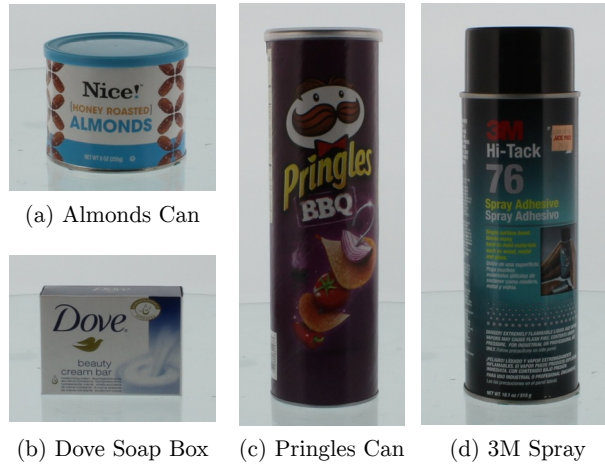
Figure 3.10: The Almonds Can, Dove Soap Box, Pringles Can, and 3M spray, which we use for quantitative measurements. We model the Almonds, Pringles, and 3M Cans using 3 cylinders: the cap, the container, and the bottom. We model the Dove Soap Box using a rectangular prism.
