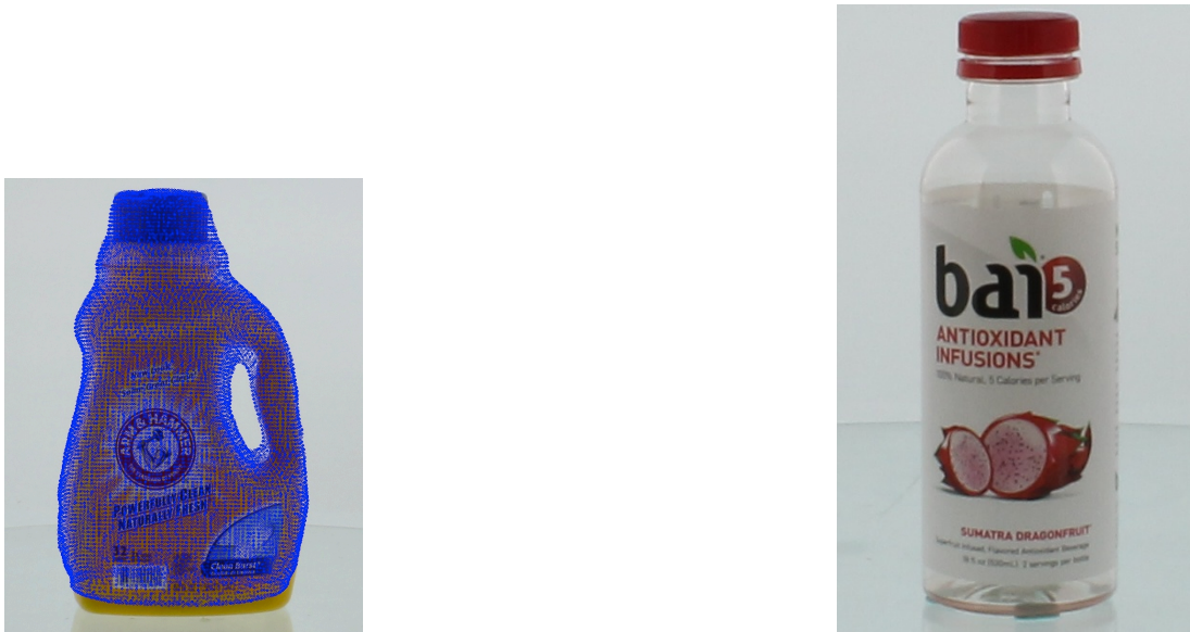
Figure 2.6: In the left image, the 3D mesh is projected onto one of the Canon images. In the right image, we show an example object for which Kinect-style RGB-D sensors yield poor-quality point clouds.
