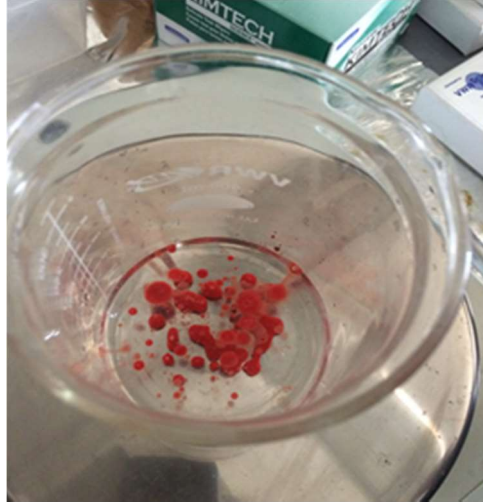
Figure 4.1.1: The manufacturer's Red Resin did not mix when placed in water
