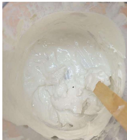
Figure 4.3.3: 27 volume % mixture when mixing the resin into the powder
