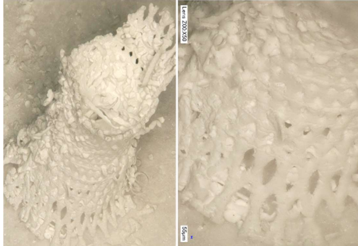
Figure 4.3.8: Sintered part made from the 6 volume % \text{Al}_2\text{O}_3 mixture with the Silmer dispersant
