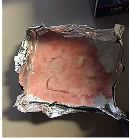
Figure 4.1.3: The Isopropyl and red resin mixture that was cured into gel-like solid
