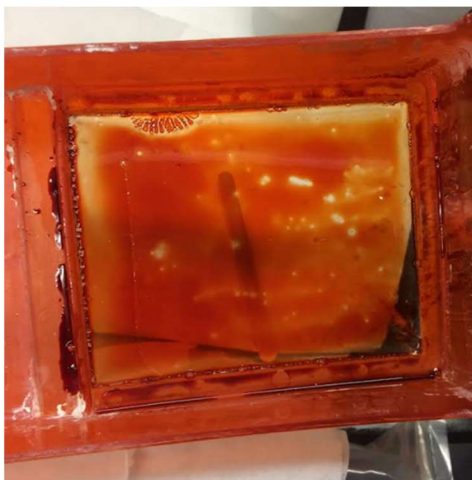
Figure 4.9.3: Cured positive photoresist coating on build area window.
