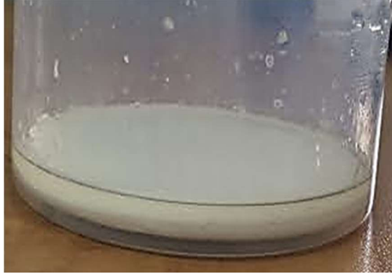
Figure 4.4.2: A 33 volume % \text{Al}_2\text{O}_3 mixture using the Dolapix dispersant with a pH of 9. The pH was in the range to disperse the powder. Separation could still be seen between the dispersed powder and the liquid phase.
