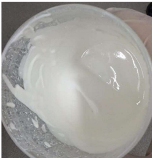
Figure 4.3.5: 18 volume % mixture when mixing the powder into the resin
