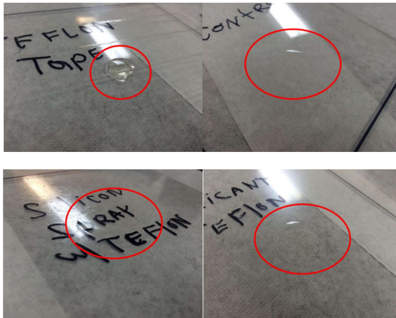
Figure 4.8.4: Photomer + Omnirad + Variquat mixture placed on the (clockwise from top-left) Teflon tape, control, silicon spray with Teflon, and lubricant with Teflon.
