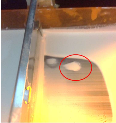
Figure 4.7.4: Cured layer sticking to the build area window.
