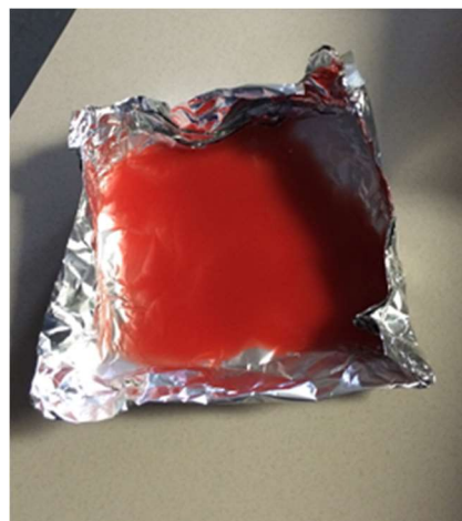
Figure 4.1.2: The ethanol and red resin mixture appeared to mix well but did not cure when exposed to
