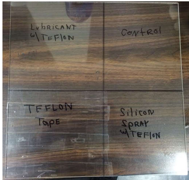
Figure 4.8.2: Sheet of acrylic glass divided into 4 areas: lubricant with Teflon, control, Teflon tape, silicon spray with Teflon.
