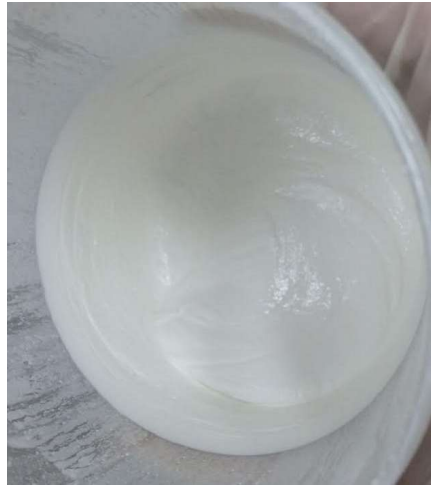
Figure 4.3.6: 27 volume % mixture when mixing the powder into the resin
