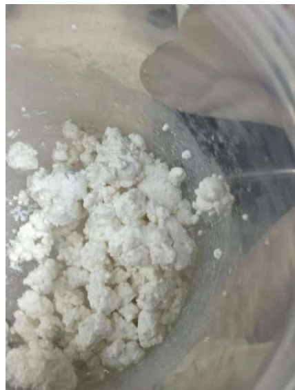
Figure 4.3.1: 50 volume % loading when mixing the resin into the powder
