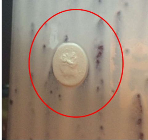
Figure 4.7.3: Printed layers stuck to the build table. The layer thickness was set to 10\mu\text{m} .
