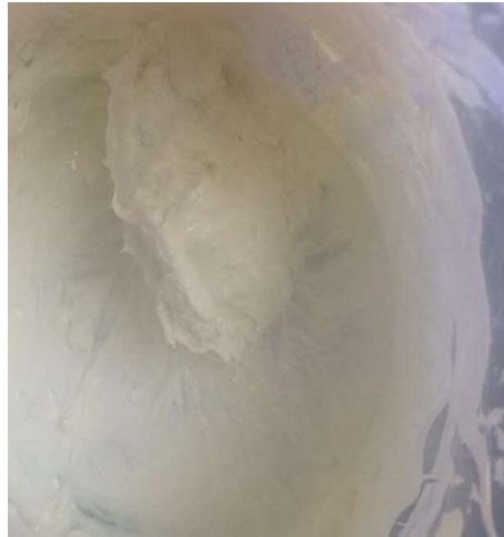
Figure 4.3.2: 36 volume % loading when mixing the resin into the powder
