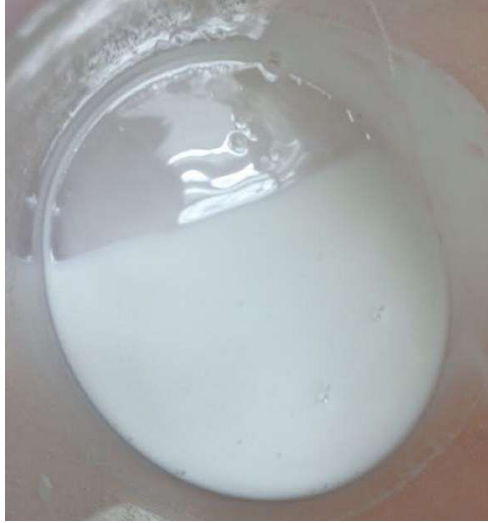
Figure 4.3.4: 6 volume % loading when mixing the powder into the resin
