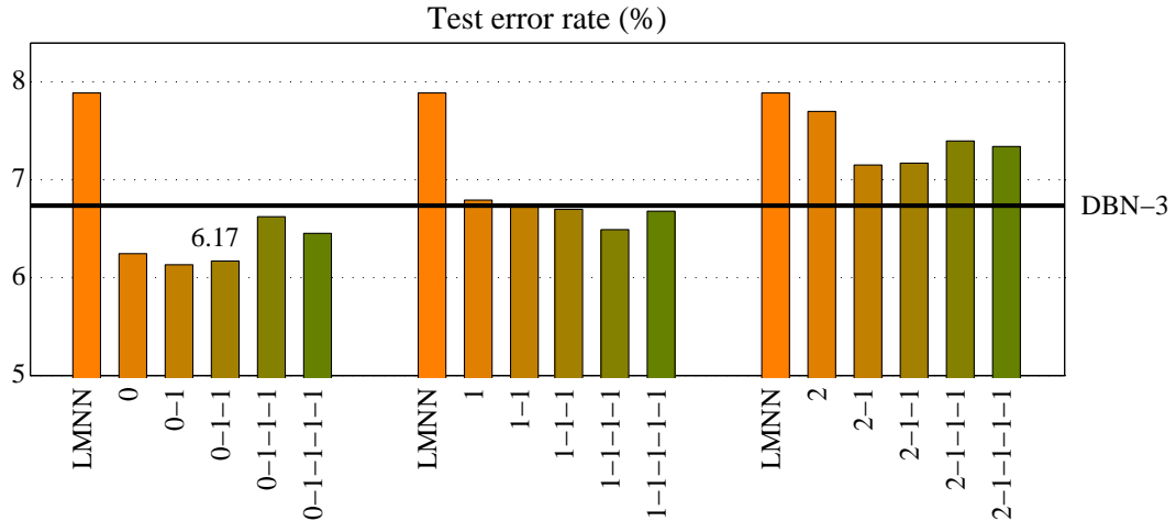
Figure 5.4: Classification error rates on the MNIST-rand data set for MKMs with different kernels and numbers of layers. The notation n_1-n_2-\dots-n_L in the horizontal axis means an MKM whose i th layer uses the arc-cosine kernel of degree n_i , while “LMNN” corresponds to the result of using LMNN with feature selection only (but without arc-cosine kernels or kernel PCA). MKMs with arc-cosine kernel have error rates from 6.13–7.69%. The error rate from the configuration that performed best on held-out set is displayed. The best previous results are 14.58% for SVMs with RBF kernels (not shown) and 6.73% for deep belief nets (Larochelle et al., 2007). See text for details.
