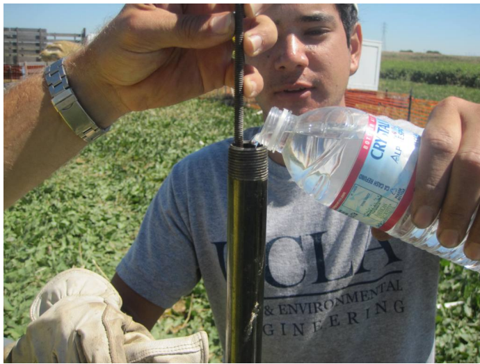
Figure 4.7. The rod is filled with water to keep suction over the sample. The all thread rod is attached to the piston at the bottom of the borehole.
