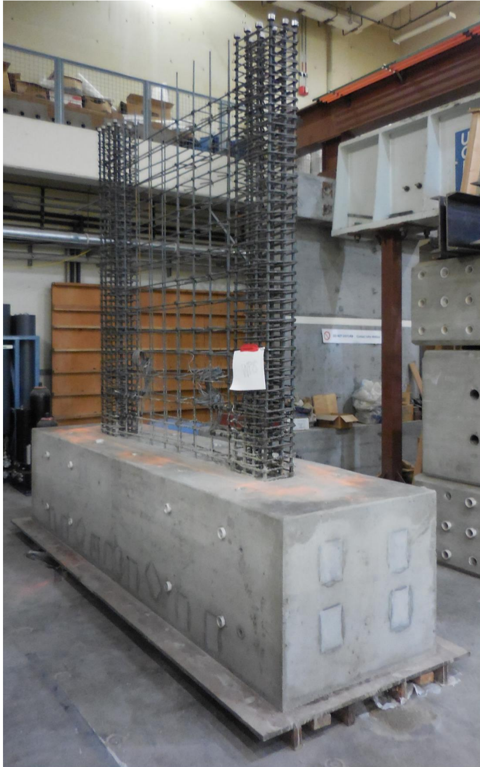
Figure 4-32: Concrete footing with wall reinforcement
