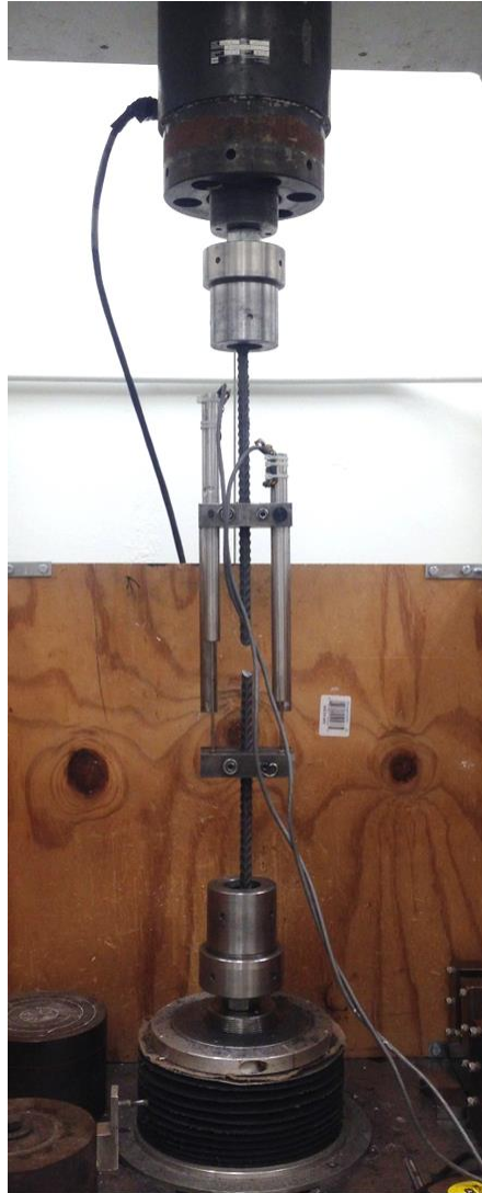
Figure 4-4: Steel reinforcement tension test setup
