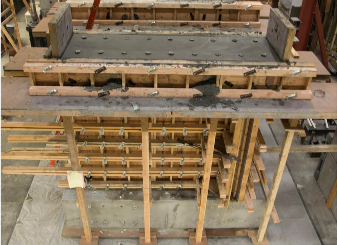
Figure 4-38: Specimen concrete curing
