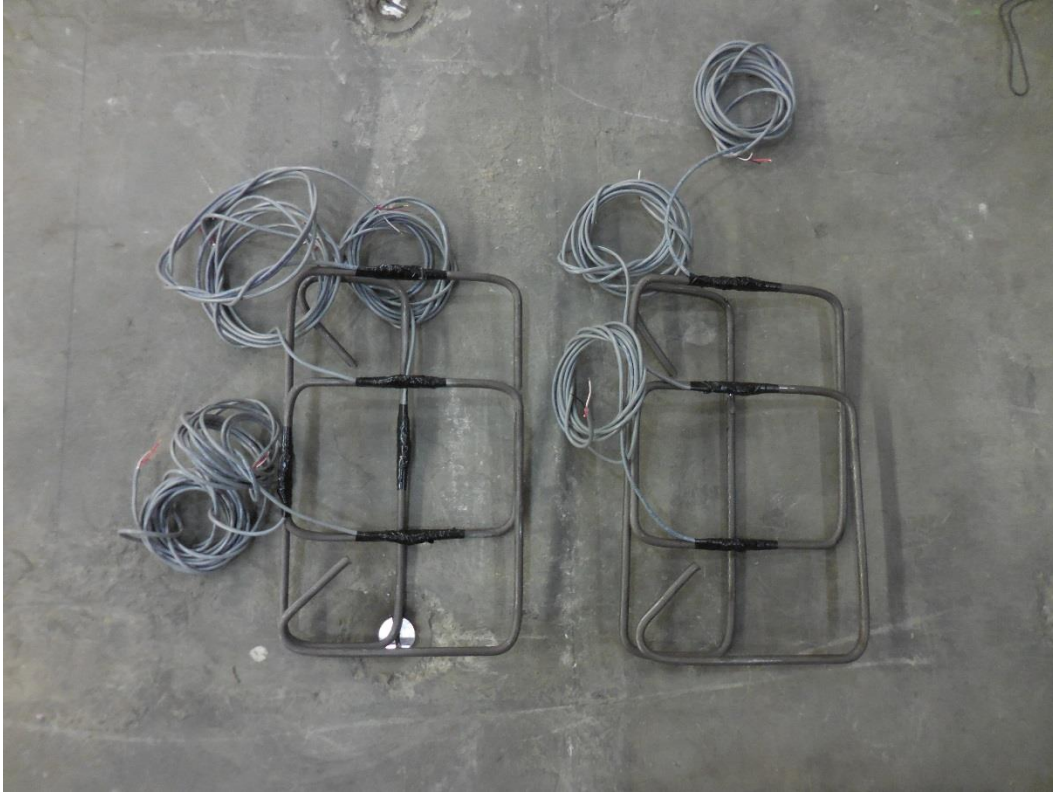
Figure 4-27: Reinforcement with strain gages installed and lead wires attached
