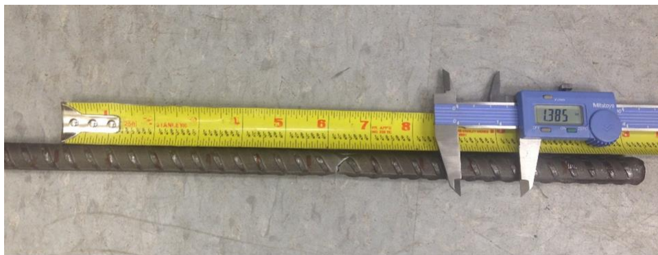
Figure 4-5: Rupture strain measurement outside gage length
