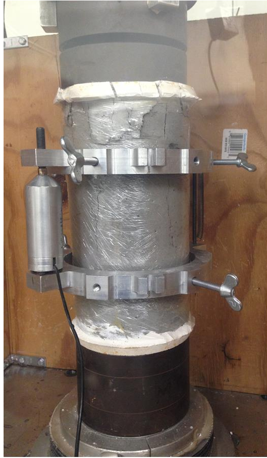
Figure 4-1: Concrete cylinder test setup
