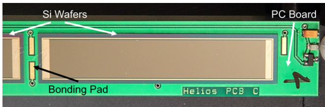
Fig. 8. Photograph of one silicon PSD mounted on a printed-circuit board as used in the HELIOS silicon-detector array.
